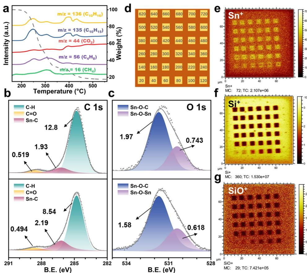
Fig. 5 (a) TGA-MS curves of **Sn4-MB**, the grey dashed line is the change in sample mass as a function of temperature; XPS for (b) C 1s and (c) O 1s XPS spectra of **Sn4-MB** after 1 hour X-ray exposure; (d) schematic illustration of the exposure dose distribution (values in  $\mu\text{C cm}^{-2}$ ); surface ToF-SIMS images of exposed **Sn4-MB** films showing (e)  $\text{Sn}^+$ , (f)  $\text{Si}^+$  (g) and  $\text{SiO}^+$  distributions.
