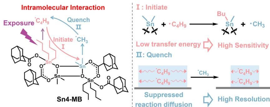
Fig. 6 Schematic exposure mechanism of **Sn4-MB** photoresist formulations.
