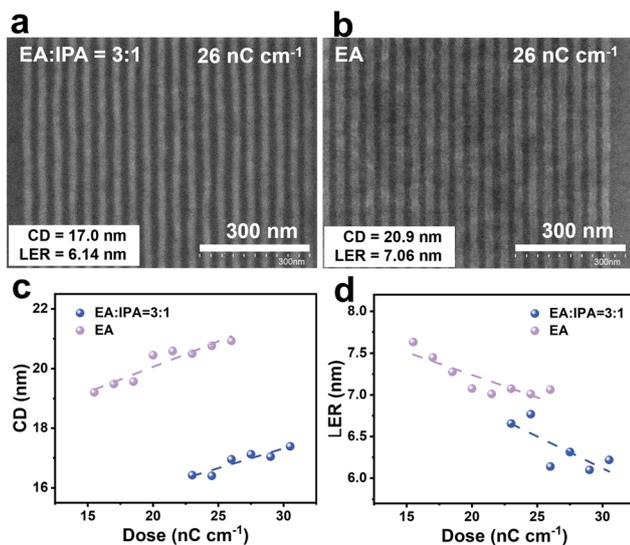
Fig. 3 SEM images of lines with a period of 40 nm at  $26 \text{ nC cm}^{-1}$  dose for thinner Sn4-MB films developed using (a) EA:IPA = 3:1 and (b) EA; relation of 40 nm pitch line (c) CD and (d) LER with dose after EA:IPA = 3:1 and EA development of thinner Sn4-MB films upon EBL line-exposure.
