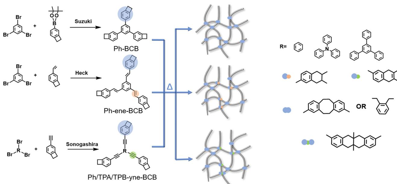
**Scheme 1** Synthesis and polymerization of tri-armed BCB-based monomers.
