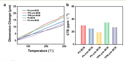
Fig. 2 TMA curves (a) and coefficient of thermal expansion (b) of cured resins.
