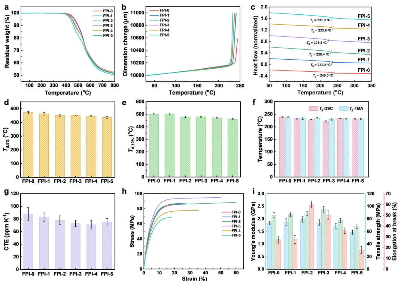
Fig. 3 Thermal and mechanical properties of FPIs. (a) TGA curves; (b) TMA curves; (c) DSC curves; (d) temperature at 5% weight loss ( $T_{d,5\%}$ ); (e) temperature at 10% weight loss ( $T_{d,10\%}$ ); (f) glass transition temperatures; (g) coefficient of thermal expansion; (h) DMA stretch curve; and (i) mechanical parameters of FPIs.
