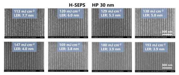
Fig. 7 SEM images of 30 nm HP patterns of the H-SEPS resist at different exposure doses by EUVL (developer: AN; film thickness: 20 nm).
