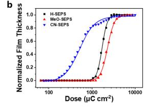
Fig. 2 (a) 3D AFM images of the H-SEPS resist pattern at different exposure doses after development in MIBK. (b) Contrast curves of X-SEPS resists
