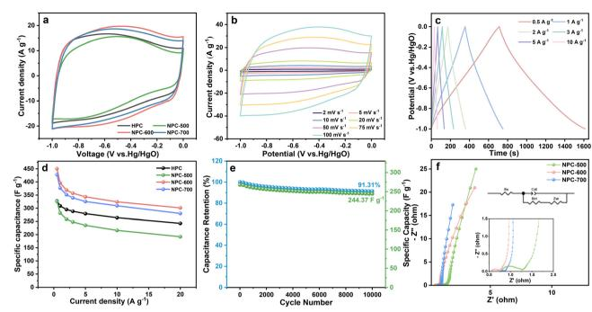
Fig. 5 (a) CV curves of HPC and NPC samples in different voltage ranges at 50 mV s $^{-1}$ ; (b) CV curves of NPC-600 at various scan rates; (c) GCD curves of NPC-600 at different current densities; (d) specific capacitance of HPC and NPC samples; (e) electrochemical stability of NPC-600 for 10 000 cycles tested at 200 mV s $^{-1}$ ; (f) Nyquist plot with an enlarged view of the high frequency region as the inset of NPCs samples.
