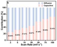
Fig. 8 (a) The b-value obtained from the linear relationship between log(i) and log(v); (b) the percentage of capacitive contributions at different scan rates of the Zn//ZnSO<sub>4</sub>//NPC-600 hybrid capacitor.
