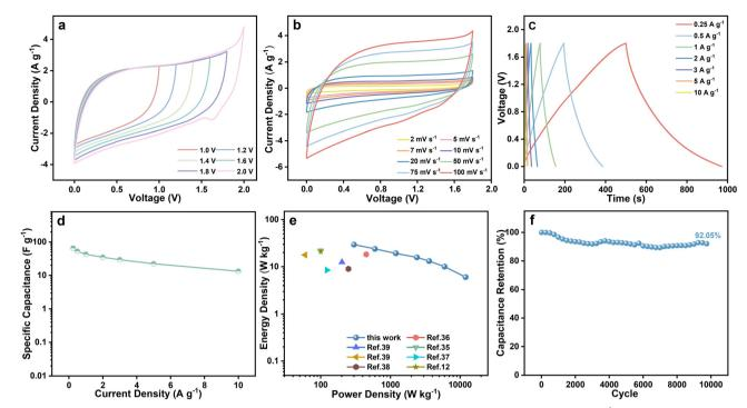
Fig. 6 (a) CV curves of the NPC-600//NPC-600 symmetrical supercapacitor in different voltage ranges at 50 mV s $^{-1}$ ; (b) CV curves of the NPC-600//NPC-600 symmetrical supercapacitor at various scan rates; (c) GCD curves of the NPC-600//NPC-600 symmetrical supercapacitor at different current densities; (d) specific capacitance of the NPC-600//NPC-600 symmetrical supercapacitor; (e) Ragone plots of the NPC-600//NPC-600 symmetrical supercapacitor for 10 000 cycles tested at 200 mV s $^{-1}$ .
