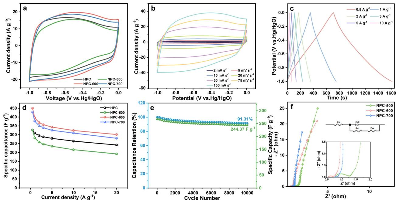
**Fig. 5** (a) CV curves of HPC and NPC samples in different voltage ranges at  $50 \text{ mV s}^{-1}$ ; (b) CV curves of NPC-600 at various scan rates; (c) GCD curves of NPC-600 at different current densities; (d) specific capacitance of HPC and NPC samples; (e) electrochemical stability of NPC-600 for 10 000 cycles tested at  $200 \text{ mV s}^{-1}$ ; (f) Nyquist plot with an enlarged view of the high frequency region as the inset of NPCs samples.
