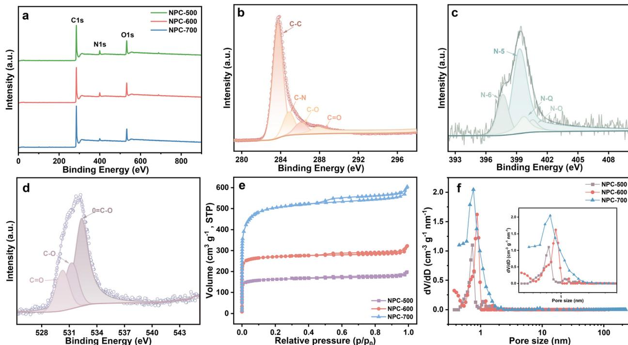
Fig. 4 (a) XPS survey spectra of NPC samples; high-resolution (b) C 1s, (c) N 1s and (d) O 1s spectra of the NPC-600 sample; (e)  $N_2$  adsorption/desorption isotherms of NPC-500, NPC-600 and NPC-700; (f) pore size distribution curves of NPC-500, NPC-600 and NPC-700 (pore size concentrated distribution area of NPCs as the inset).
