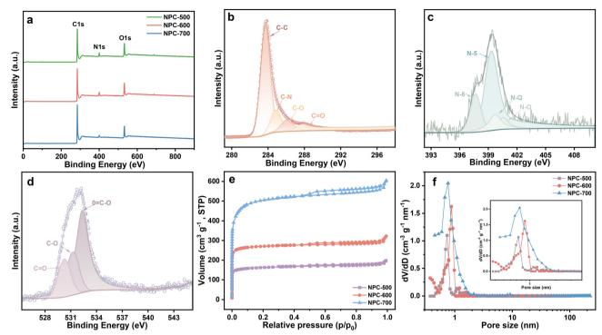
Fig. 4 (a) XPS survey spectra of NPC samples; high-resolution (b) C 1s, (c) N 1s and (d) O 1s spectra of the NPC-600 sample; (e) N₂ adsorption/ desorption isotherms of NPC-500, NPC-600 and NPC-700; (f) pore size distribution curves of NPC-500, NPC-600 and NPC-700 (pore size concentrated distribution area of NPCs as the inset).
