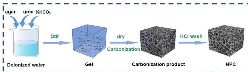
Fig. 1 Schematic illustration of the synthesis of NPC samples.
