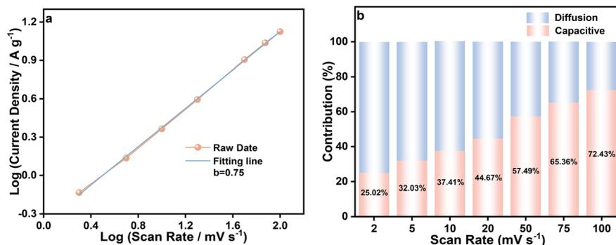
Fig. 8 (a) The *b*-value obtained from the linear relationship between log(*i*) and log(*v*); (b) the percentage of capacitive contributions at different scan rates of the Zn//ZnSO<sub>4</sub>//NPC-600 hybrid capacitor.
