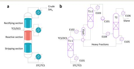
Fig. 8 Reactive distillation (RD) based silane production process from chlorosilanes. (a) Main configuration of the RD column; (b) conceptual design for process simulation.
