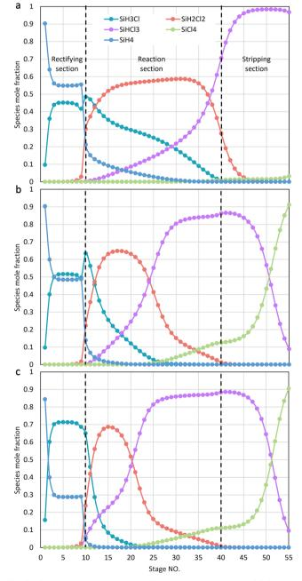
Fig. 5 Species mole fraction profiles in the vapor phase. (a) Scheme IV; (b) scheme III; (c) scheme II.
