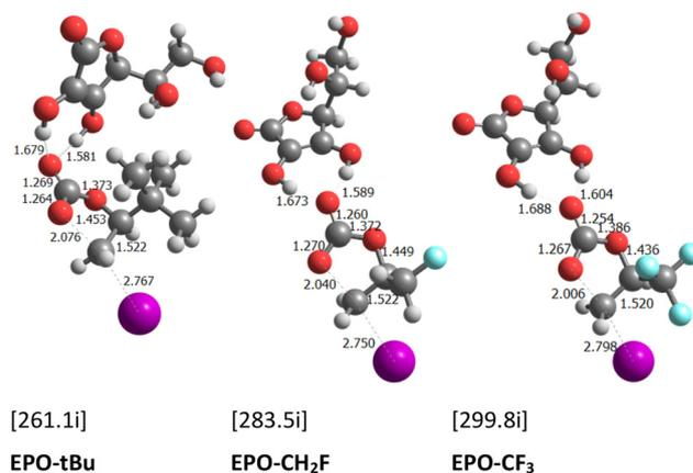
Fig. 2 Transition state **TS-CD** of the cycloaddition of  $CO_2$  for **EPO-*t*Bu**, **EPO-CH<sub>2</sub>F** and **EPO-CF<sub>3</sub>** (selected distances in Å and imaginary frequencies included within brackets in cm<sup>-1</sup>).
