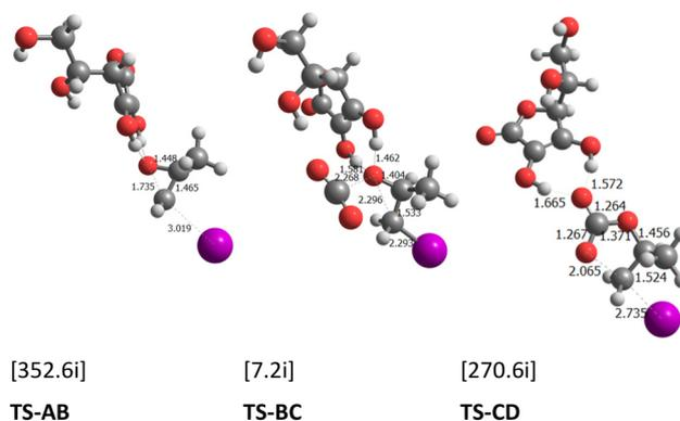
**Fig. 1** Transition states of the cycloaddition of carbon dioxide (CO<sub>2</sub>) to epoxide **EPO-CH<sub>3</sub>** (selected distances in Å and imaginary frequencies included within brackets in cm<sup>-1</sup>).
