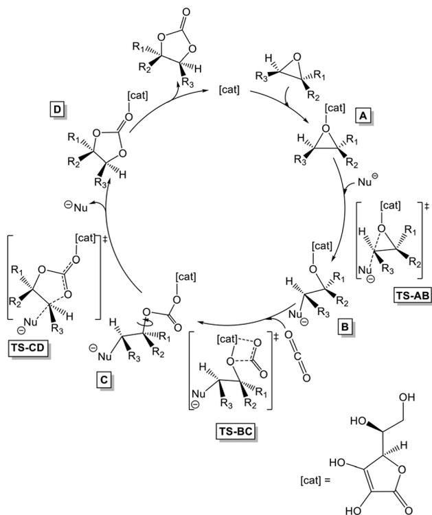
**Scheme 1** Cycloaddition of epoxides (R = substituent; cat = ascorbic acid; Nu = nucleophile, being F, Cl, Br, I, or TBAI) and CO<sub>2</sub>.
