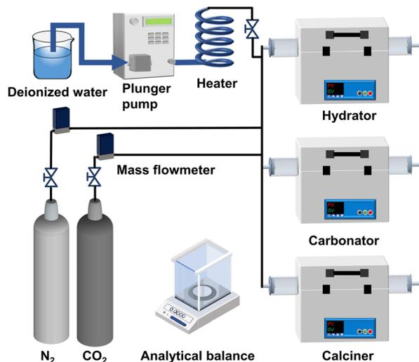
Fig. 12 Diagram of the dual-packed bed reactor.
