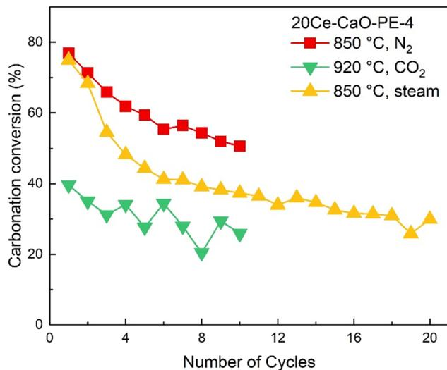
Fig. 7 Reactivity of 20Ce-CaO-PE-4 under different calcination conditions in the dual-packed bed reactor. Reaction conditions: calcination: 10 min; carbonation: 15% CO<sub>2</sub>, 85% N<sub>2</sub>, 650 °C, 15 min.
