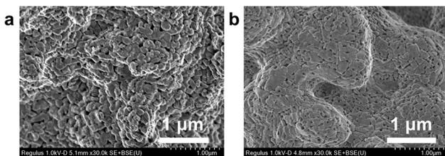
**Fig. 11** SEM images of (a) spent 20Ce-CaO-PE-4 and (b) spent CaO-PE-4 after ten cycles in the dual-packed bed reactor. Reaction conditions: calcination: N<sub>2</sub>, 850 °C, 10 min; carbonation: 15% CO<sub>2</sub>, 10% steam, 75% N<sub>2</sub>, 650 °C, 15 min.
