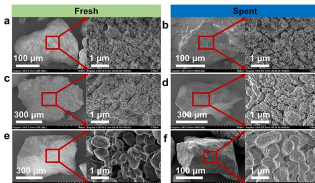
Fig. 6 SEM images of the CeO<sub>2</sub>-doped and undoped CaO-based pellets before and after ten cycles measured in the dual-packed bed reactor. (a) Fresh and (b) spent 20Ce-CaO-PE-1; (c) fresh and (d) spent 20Ce-CaO-PE-4; (e) fresh and (f) spent CaO-PE-4.
