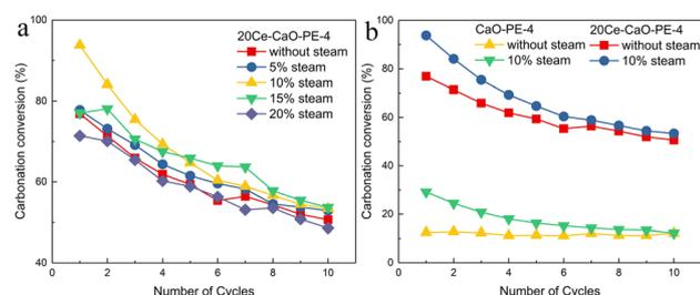
Fig. 10 Reactivity of (a) 20Ce-CaO-PE-4 and (b) CaO-PE-4 at varying concentrations of steam during carbonation in the dual-packed bed reactor. Reaction conditions: calcination:  $N_2$ , 850 °C, 10 min; carbonation: 15%  $CO_2$  (balanced with  $N_2$ ), 650 °C, 15 min.
