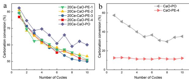
Fig. 5 Reactivity of the (a) CeO<sub>2</sub>-doped and (b) undoped CaO-based pellets sieved to different particle sizes in the dual-packed bed reactor. Particle size had minimal impact on the performance of CeO<sub>2</sub>-doped CaO-based pellets. Reaction conditions: calcination: N<sub>2</sub>, 850 °C, 10 min; carbonation: 15% CO<sub>2</sub>, 85% N<sub>2</sub>, 650 °C, 15 min.
