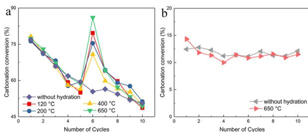
Fig. 8 Reactivity of (a) 20Ce-CaO-PE-4 and (b) CaO-PE-4 hydrated under different temperatures in the dual-packed bed reactor. Reaction conditions: calcination: N<sub>2</sub>, 850 °C, 10 min; carbonation: 15% CO<sub>2</sub>, 85% N<sub>2</sub>, 650 °C, 15 min; hydration: 100% steam, 60 min.
