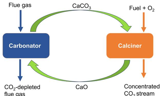
Fig. 1 Illustration of the CaL technology for capturing CO<sub>2</sub> from the flue gas.
