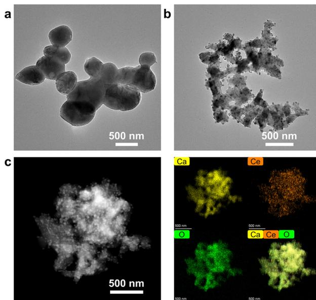
**Fig. 3** HAADF-STEM images and EDX mapping of fresh CaO-PO and 20Ce-CaO-PO. (a) HAADF-STEM image of CaO-PO; (b) HAADF-STEM image and (c) EDX mapping of 20Ce-CaO-PO. CeO<sub>2</sub> effectively reduces the grain size.
