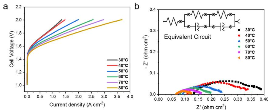
Fig. 9 (a) Linear sweep voltammograms in the range of 30–80 °C of the AEM-WE cell based on the  $\text{Ni}_{0.75}\text{Fe}_{0.25}\text{O}$  electrocatalyst at the anode; (b) electrochemical impedance spectroscopy plots (Nyquist), recorded at 1.8 V. The equivalent circuit of the EIS is shown in Fig. 9b.
