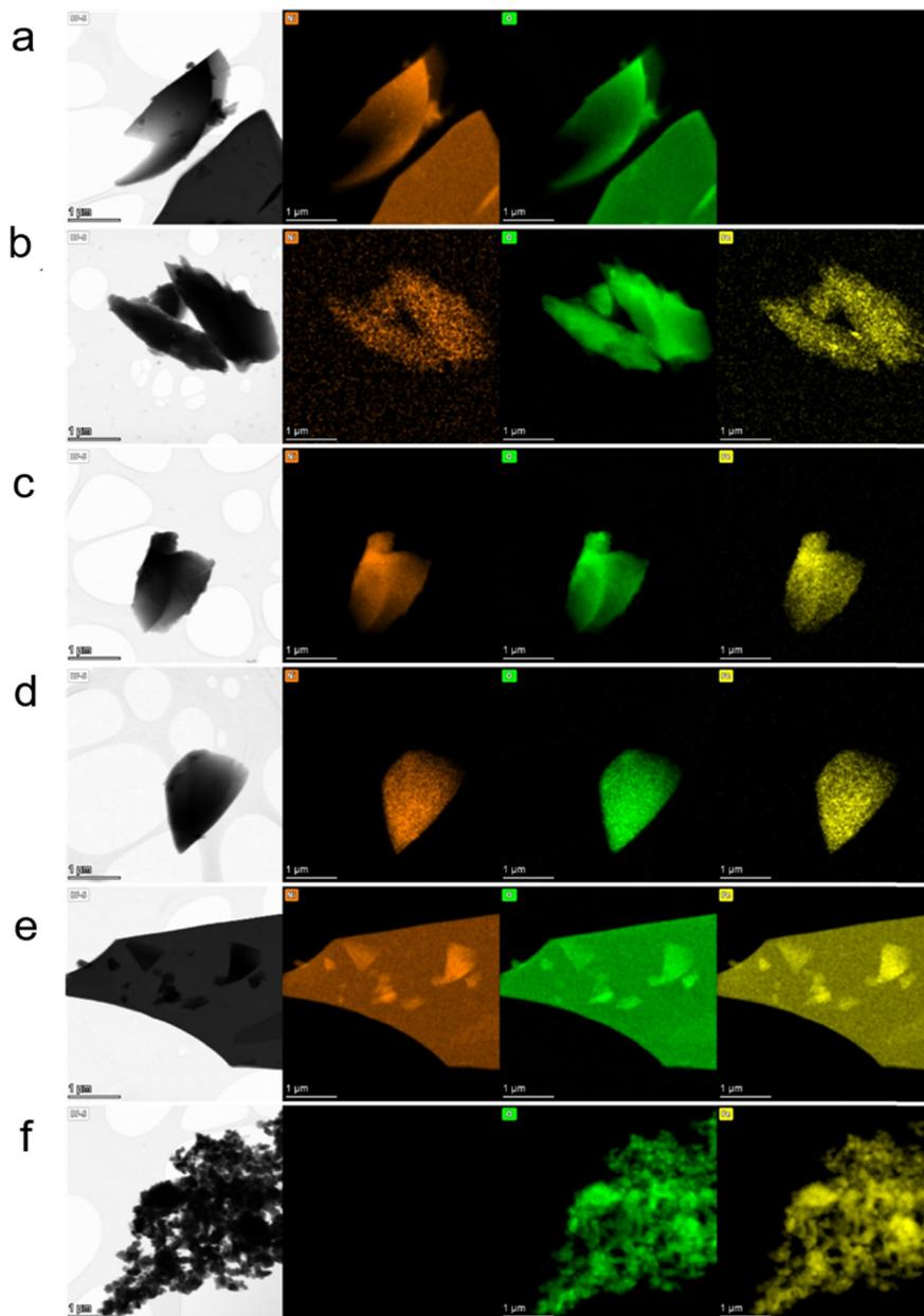
Fig. 5 STEM images of samples (a)  $\text{Ni}_1\text{Fe}_0\text{O}$ , (b)  $\text{Ni}_{0.995}\text{Fe}_{0.005}\text{O}$ , (c)  $\text{Ni}_{0.95}\text{Fe}_{0.05}\text{O}$ , (d)  $\text{Ni}_{0.75}\text{Fe}_{0.25}\text{O}$ , (e)  $\text{Ni}_{0.50}\text{Fe}_{0.50}\text{O}$  and (f)  $\text{Ni}_0\text{Fe}_1\text{O}$ . From left to right columns: STEM bright field images, Ni map, O map, and Fe map.
