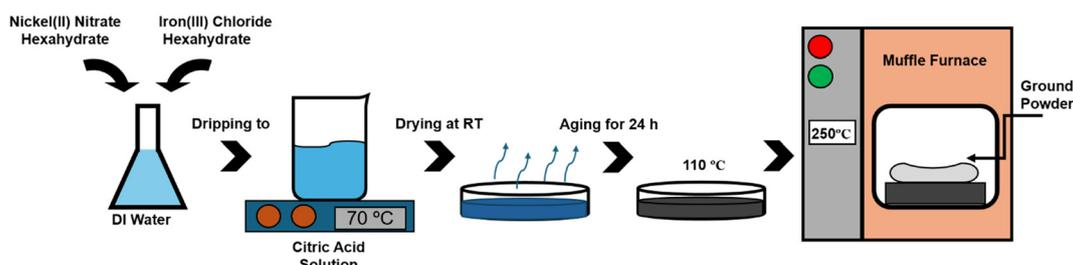
**Fig. 1** Schematic illustration of NiFe oxide synthesis.
