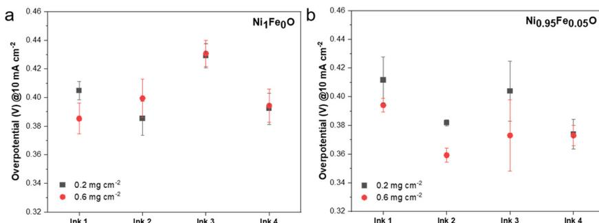
Fig. 6 OER overpotentials of (a)  $\text{Ni}_1\text{Fe}_0\text{O}$  and (b)  $\text{Ni}_{0.95}\text{Fe}_{0.05}\text{O}$  measured at  $10 \text{ mA cm}^{-2}$ . The effect of different ink formulations on the OER electrocatalytic activity is reported.
