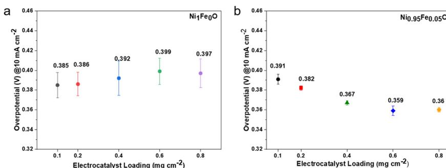
Fig. 7 Overpotentials of (a)  $\text{Ni}_1\text{Fe}_0\text{O}$  and (b)  $\text{Ni}_{0.95}\text{Fe}_{0.05}\text{O}$  measured at  $10 \text{ mA cm}^{-2}$ . The effect of different electrocatalyst loadings on the OER electrocatalytic activity is reported.
