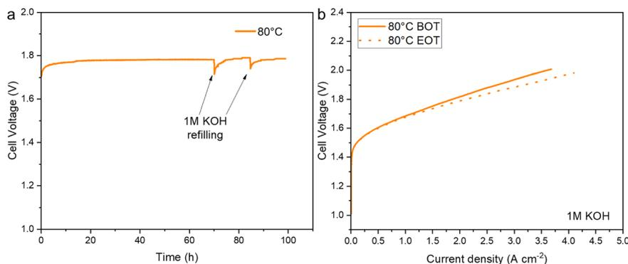
**Fig. 10** (a) Chronopotentiometric curve at 80 °C, in 1 M KOH solution and at 1 A cm<sup>-2</sup> of the cell based on the Ni<sub>0.75</sub>Fe<sub>0.25</sub>O electrocatalyst at the anode; (b) linear sweep voltammetric curves at the beginning of the test (BOT) and at the end of the test (EOT).
