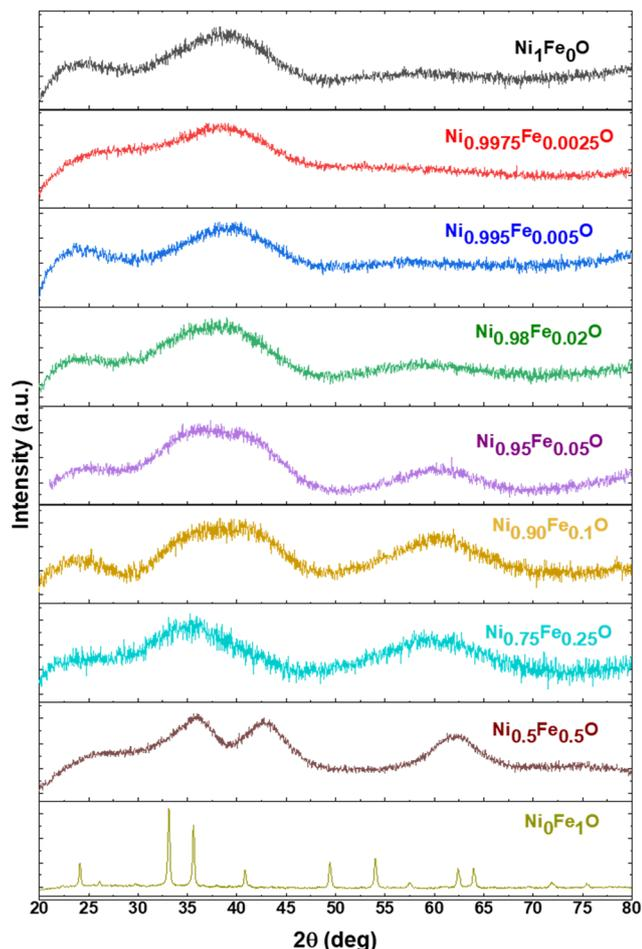
Fig. 2 XRD diffractograms of the synthesized NiFe oxides.
