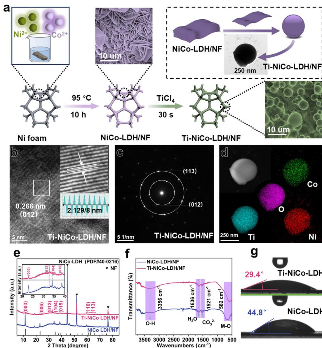
**Fig. 1** (a) Schematic diagram of the process of exfoliating NiCo-LDH/NF nanosheets with TiCl<sub>4</sub>; (b) HRTEM image of Ti-NiCo-LDH/NF; (c) SAED pattern of Ti-NiCo-LDH/NF; (d) energetic elemental mapping of Ni, Co, Ti, and O; (e) XRD spectra; (f) FTIR spectra of Ni-LDH/NF and Ti-NiCo-LDH/NF; (g) contact angles of Ni-LDH/NF and Ti-NiCo-LDH/NF.
