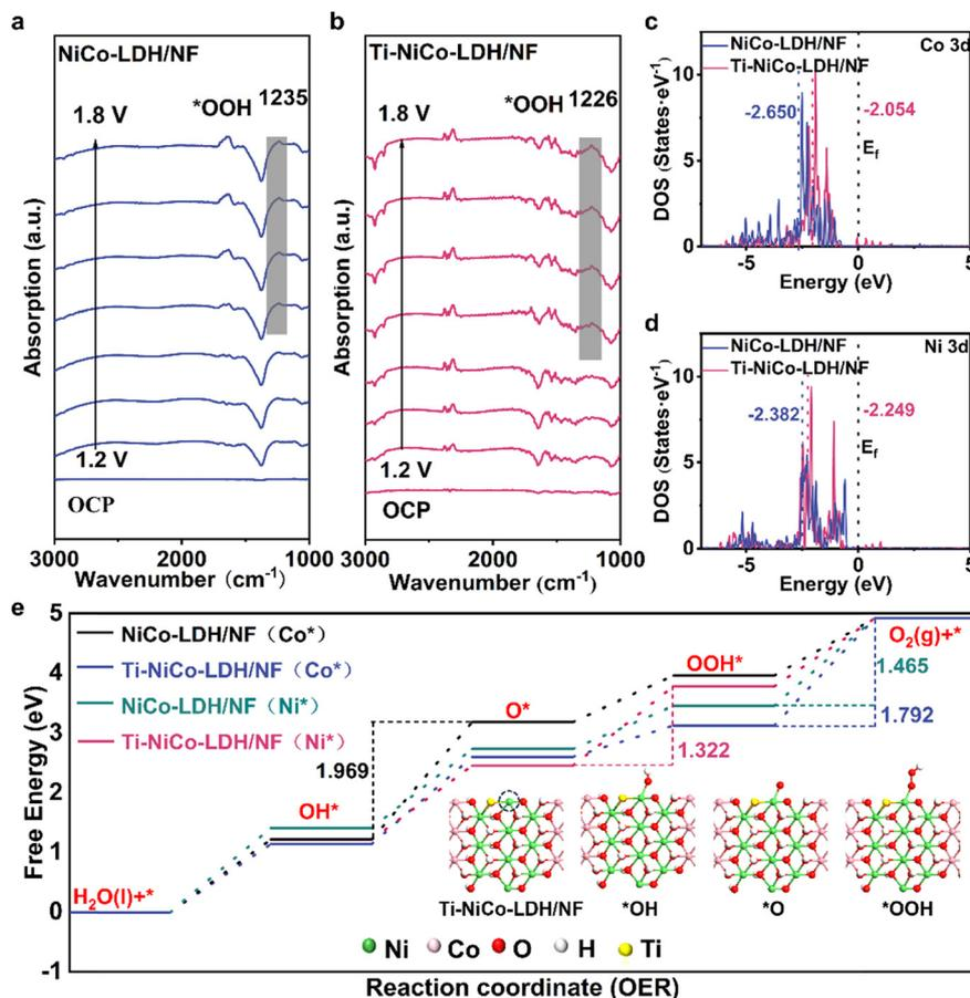
Fig. 4 *In situ* spectroscopic characterization: (a) NiCo-LDH/NF; (b) Ti-NiCo-LDH/NF; (c and d) the calculated DOS of NiCo-LDH/NF and Ti-NiCo-LDH/NF; (e) the OER free energy diagram for AEM steps and optimized intermediate geometry for Ni sites of Ti-NiCo-LDH/NF (inset).
