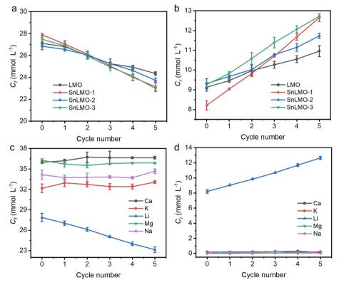
Fig. 6 Concentration changes of Li<sup>+</sup> in feed solution (a), corresponding recovery solution (b), simulated brine (c), and corresponding recovery solution (d) during lithium intercalation or deintercalation.
