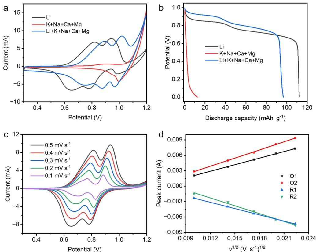
Fig. 3 Cyclic voltammograms curve (a) and discharge curves (b) of SnLMO-1 in different electrolytes; cyclic voltammograms curve of SnLMO-1 in different scan rate (c); linear relationship between  $v^{1/2}$  and corresponding with redox peak current (d).
