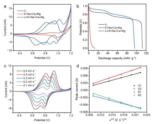
Fig. 3 Cyclic voltammograms curve (a) and discharge curves (b) of SnLMO-1 in different electrolytes; cyclic voltammograms curve of SnLMO-1 in different scan rate (c); linear relationship between  $v^{1/2}$  and corresponding with redox peak current (d).
