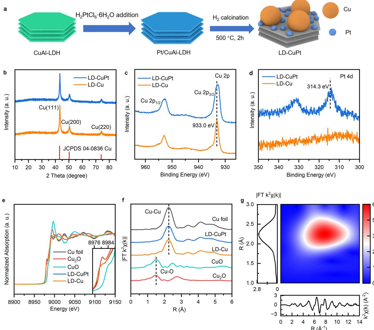
**Fig. 1** (a) Schematic diagram of the synthesis of LD-CuPt. (b) XRD patterns of LD-CuPt, and LD-Cu. (c) XPS Cu 2p spectra of LD-CuPt and LD-Cu. (d) XPS Pt 4d spectra of LD-CuPt, and LD-Cu, (e) Cu K-edge X-ray absorption near-edge structure for LD-CuPt, LD-Cu, and reference samples. (f) Cu K-edge EXAFS spectra of LD-CuPt, LD-Cu and reference samples. (g) Wavelet transform for the  $k^2$ -weighted EXAFS signal of LD-CuPt.
