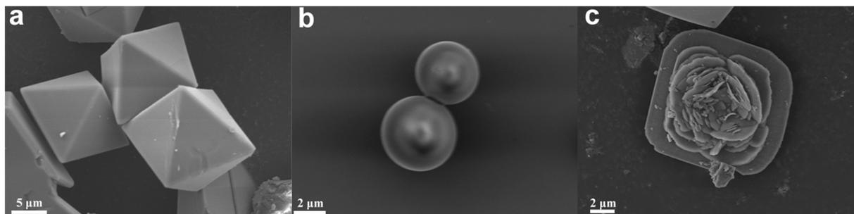
Fig. 1 SEM images of (a) HKUST-1, (b) SBA-16, and (c) HK@SB-1 (1 wt% SBA-16 modified HKUST-1).
