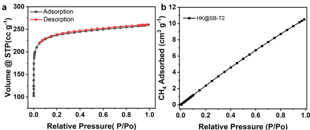
Fig. 7 (a) Isothermal N<sub>2</sub> adsorption and desorption curves and (b) CH<sub>4</sub> adsorption performance of HK@SB-T2.
