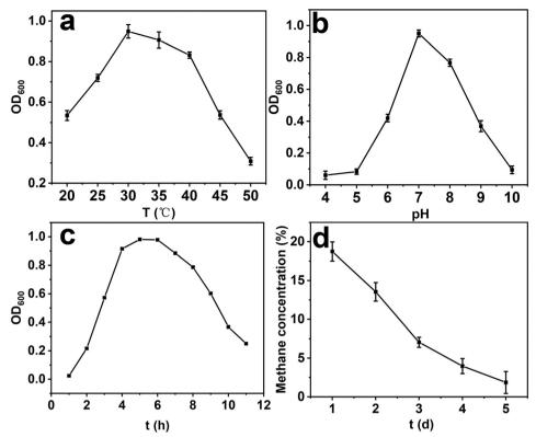
Fig. 5 (a) Effect of temperature, and (b) pH on the growth of *methanotroph*; (c) the growth curve of the *methanotrophs* under optimal conditions; (d) changes in methane content during the growth of *methanotroph*.
