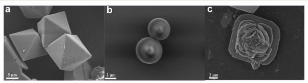
Fig. 1 SEM images of (a) HKUST-1, (b) SBA-16, and (c) HK@SB-1 (1 wt% SBA-16 modified HKUST-1).
