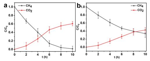
Fig. 9 Changes in  $CH_4$  and  $CO_2$  in the (a) HK@SB-T2 and (b) free cell methane degradation system (gas composition in the reactor was analyzed using gas chromatography every 2 hours). Error bars indicate the standard deviations of three independent experiments.
