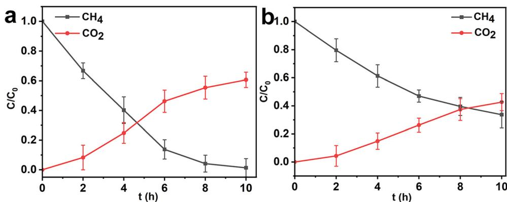
**Fig. 9** Changes in CH<sub>4</sub> and CO<sub>2</sub> in the (a) HK@SB-T2 and (b) free cell methane degradation system (gas composition in the reactor was analyzed using gas chromatography every 2 hours). Error bars indicate the standard deviations of three independent experiments.
