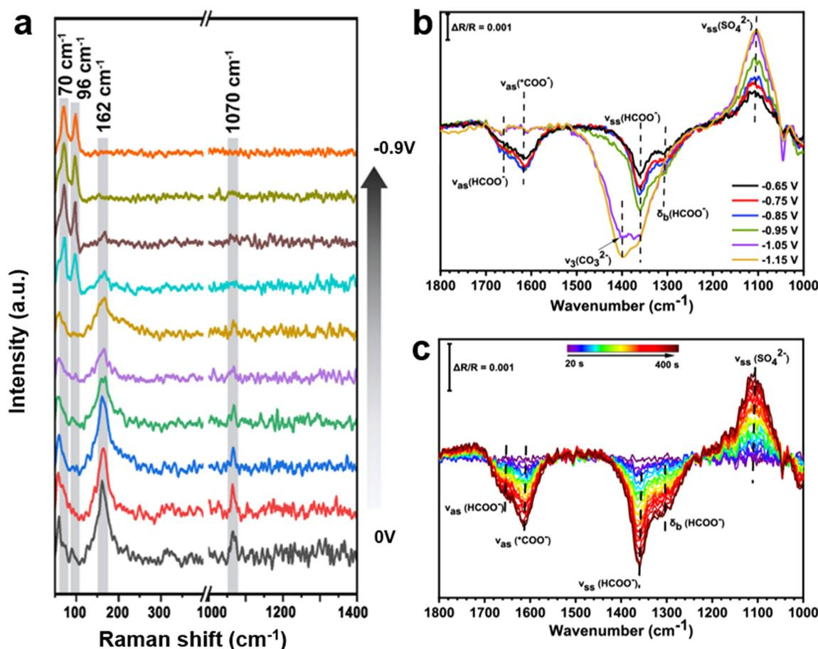
Fig. 7 (a) *In situ* Raman spectra for the transformation of the  $\text{Bi}_2\text{O}_3$  precursor from  $\text{Bi}_2\text{O}_2\text{CO}_3$  to Bi during the  $\text{CO}_2\text{RR}$ <sup>38</sup> (copyright 2022 American Chemical Society); potential-dependent (b) and time-dependent (c) IR spectra measured in a  $\text{CO}_2$ -saturated  $0.1\text{ M K}_2\text{SO}_4$  solution for the ZnBi-3 electrode<sup>86</sup> (copyright 2024 American Chemical Society).
