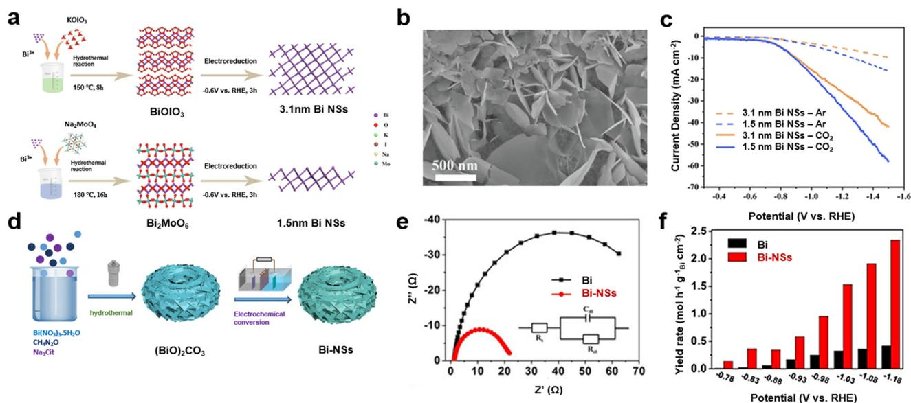
**Fig. 1** (a) Schematic of the preparation of ultrathin Bi NSs; (b) SEM image of 1.5 nm Bi NSs; (c) LSV curves for 3.1 nm Bi NSs and 1.5 nm Bi NSs in a CO<sub>2</sub> and Ar saturated 0.5 M KHCO<sub>3</sub> solution<sup>36</sup> (copyright 2023 Elsevier); (d) schematic of the preparation of Bi NSs; (e) Nyquist plots and (f) formate yielded rates for CO<sub>2</sub>RR over Bi NSs and Bi nanopowders<sup>35</sup> (copyright 2021 John Wiley and Sons).
