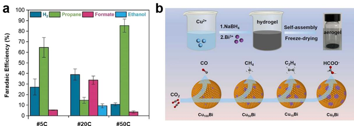
Fig. 6 (a) Faradaic efficiencies of CO<sub>2</sub>RR on CuBi catalysts prepared with different charge values passed through the substrate using 0.1 M KHCO<sub>3</sub> catholyte<sup>92</sup> (copyright 2022 Elsevier); (b) schematic of synthesis procedure for Cu<sub>x</sub>Bi aerogels and different product selectivity<sup>32</sup> (copyright 2022 Elsevier).
