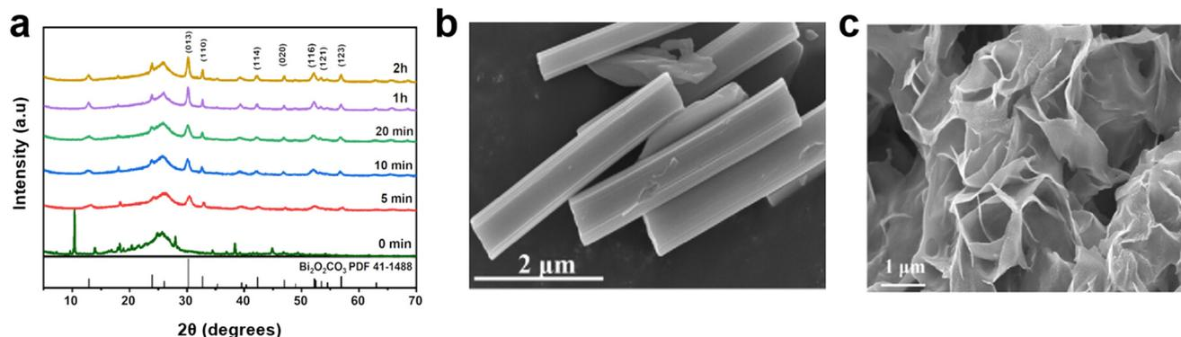
**Fig. 2** (a) XRD patterns of Bi-BTC after different electrolysis times (0 min, 5 min, 10 min, 20 min, 1 h, and 2 h); SEM image of Bi-BTC (b) before and (c) following electrolysis<sup>57</sup> (copyright 2024 American Chemical Society).
