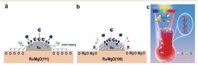
Fig. 2 Hydrogen diffusion over (a) Ru/MgO(111) and (b) Ru/MgO(100) exhibits distinct characteristics. <sup>16</sup> Copyright 2023, Nature Publishing Group. (c) Illustration of the cooperative action of charge carriers and photo-induced thermal energy in accelerating the removal of ammonia on Ru NPs/ GaN NWs/Si.<sup>17</sup> Copyright 2024, Nature Publishing Group.
