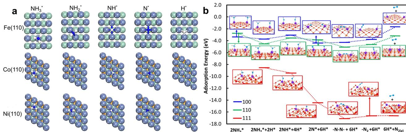
Fig. 5 (a) Fe(110), Co(111) and Ni(111) surfaces exhibit the most stable  $\text{NH}_x$  ( $x = 0-3$ ) and H adsorption arrangements.<sup>46</sup> Re-drawing from ref. 46. Copyright 2012, Elsevier. (b) At MgO-supported twin Ru single atoms, energy patterns and their related optimized intermediate structures for ammonia decomposition and N–N recombination routes to generate  $\text{N}_2$  are shown.<sup>16</sup> Copyright 2023, Nature Publishing Group.
