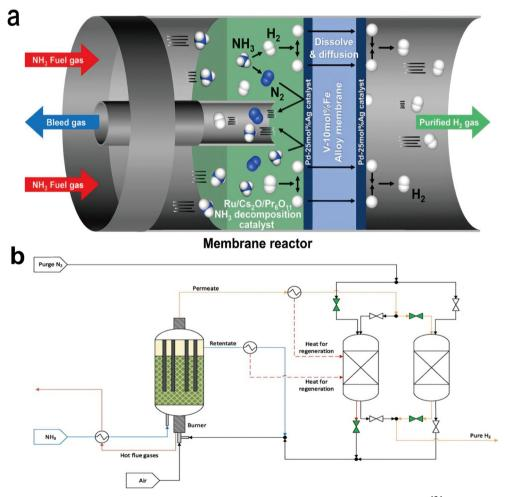
Fig. 12 (a) The membrane reactor for separating and purifying hydrogen from  $NH_3$  gas is shown schematically. <sup>124</sup> Copyright 2022, Elsevier. (b) The ammonia-based hydrogen generation system is put up for experimental purposes. <sup>131</sup> Copyright 2022, Elsevier.
