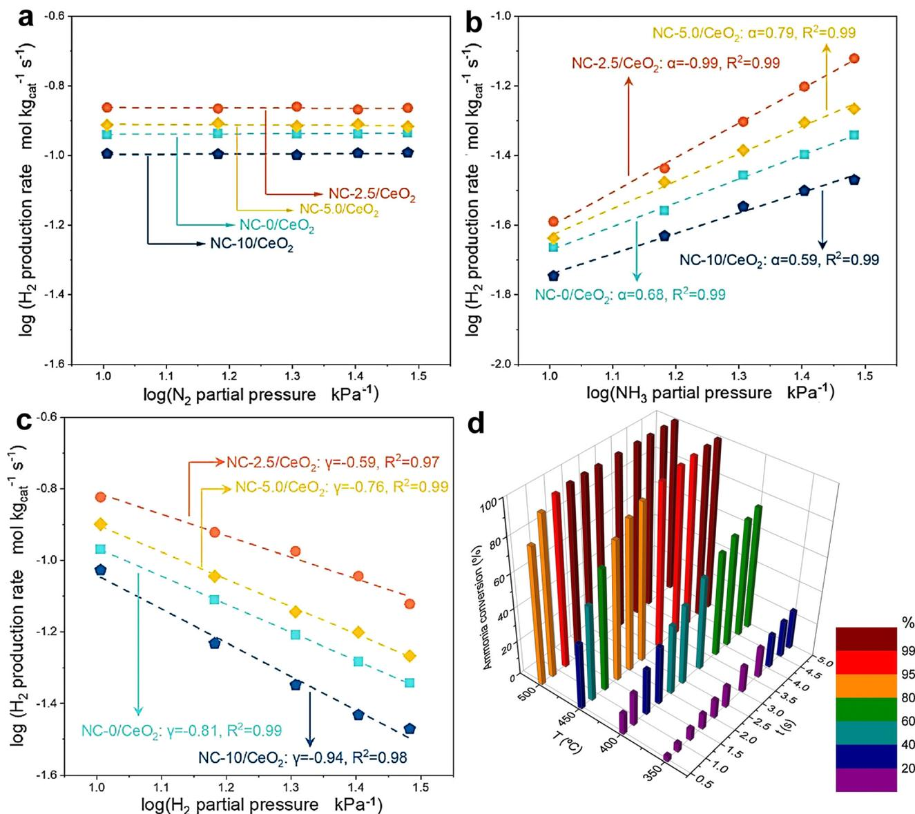
Fig. 3 Determining the exact order of reaction for (a)  $N_2$ , (b)  $NH_3$ , and (c)  $H_2$  using kinetics graphs.<sup>31</sup> Copyright 2023, Elsevier. (d) Results from a mathematical model of ammonia decomposition on  $2.5Ni0.5Ru/CeO_2$  under different temperatures and interaction periods with dry ammonia.<sup>32</sup> Copyright 2021, Elsevier.
