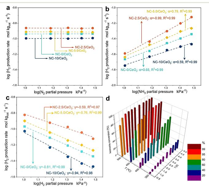
Fig. 3 Determining the exact order of reaction for (a) N<sub>2</sub>, (b) NH<sub>3</sub>, and (c) H<sub>2</sub> using kinetics graphs. Topyright 2023, Elsevier. (d) Results from a mathematical model of ammonia decomposition on 2.5Ni0.5Ru/CeO<sub>2</sub> under different temperatures and interaction periods with dry ammonia.<sup>32</sup> Copyright 2021, Elsevier.
