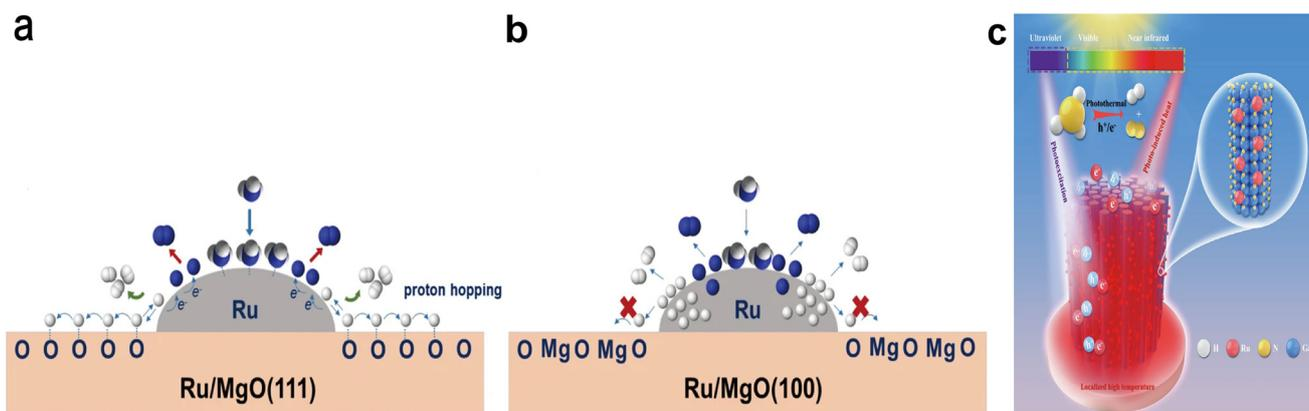
Fig. 2 Hydrogen diffusion over (a) Ru/MgO(111) and (b) Ru/MgO(100) exhibits distinct characteristics.<sup>16</sup> Copyright 2023, Nature Publishing Group. (c) Illustration of the cooperative action of charge carriers and photo-induced thermal energy in accelerating the removal of ammonia on Ru NPs/GaN NWs/Si.<sup>17</sup> Copyright 2024, Nature Publishing Group.
