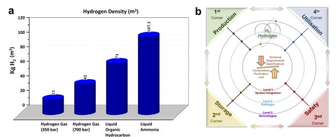
Fig. 1 (a) Density comparison of several kinds of hydrogen storage.<sup>3</sup> Copyright 2023, Royal Society of Chemistry. (b) The four-cornered model suggesting a hydrogen square.4 Copyright 2020, Elsevier.
