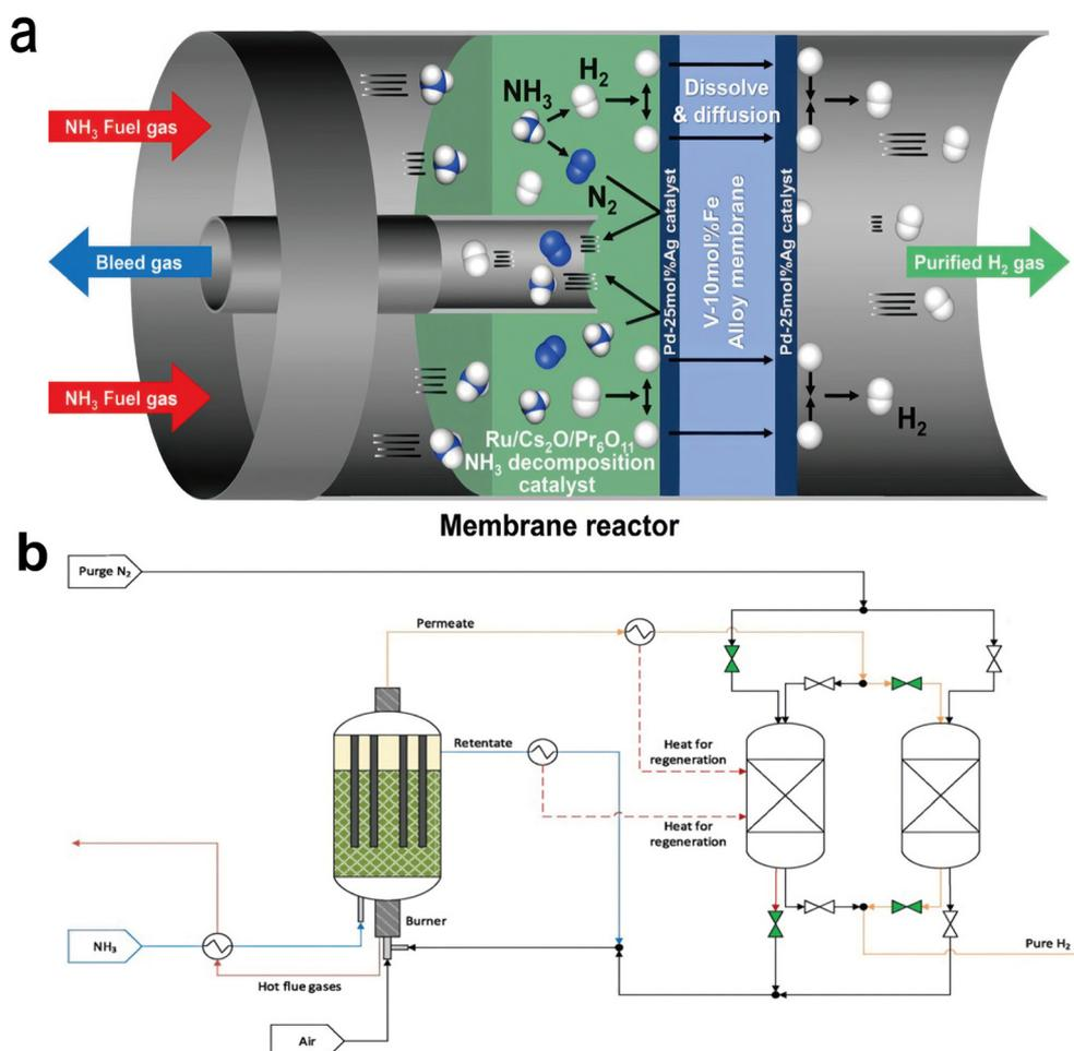
Fig. 12 (a) The membrane reactor for separating and purifying hydrogen from  $\text{NH}_3$  gas is shown schematically.<sup>124</sup> Copyright 2022, Elsevier. (b) The ammonia-based hydrogen generation system is put up for experimental purposes.<sup>131</sup> Copyright 2022, Elsevier.
