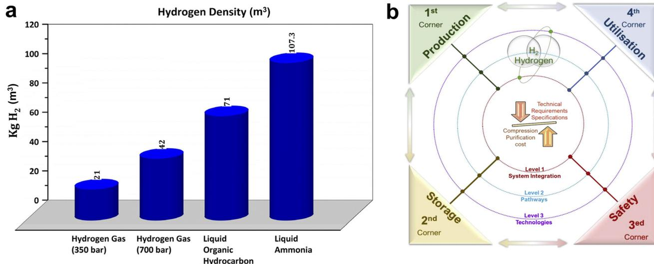
Fig. 1 (a) Density comparison of several kinds of hydrogen storage.<sup>3</sup> Copyright 2023, Royal Society of Chemistry. (b) The four-cornered model suggesting a hydrogen square.<sup>4</sup> Copyright 2020, Elsevier.
