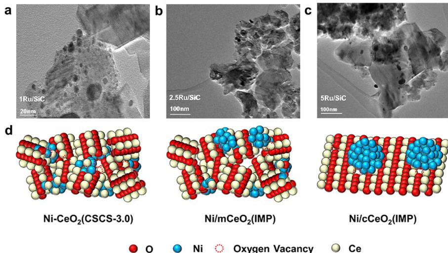
**Fig. 9** Ru catalysts supported by SiC. (a) 2.5 Ru/SiC, (b) 2.5Ru/SiC and (c) 5Ru/SiC reduced at 673 K are shown in TEM pictures.<sup>80</sup> Re-drawing from ref. 80. Copyright 2021, Elsevier. (d) Modelling of the structures of Ni-CeO<sub>2</sub>(CSCS-3.0), Ni/mCeO<sub>2</sub>(IMP), and Ni/cCeO<sub>2</sub>(IMP).<sup>82</sup> Copyright 2023, Elsevier.
