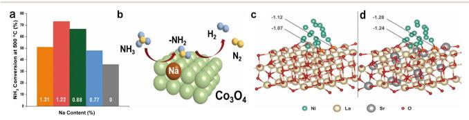
Fig. 8 (a) Comparison of ammonia decomposition rates via Na-doped Co<sub>3</sub>O<sub>4</sub> and Co<sub>3</sub>O<sub>4</sub>-CA. (b) Diagrammatic representation of the catalyst surface ammonia decomposition process.<sup>66</sup> Copyright 2023, Elsevier. Ni/La<sub>2</sub>O<sub>3</sub> (c) and Ni/Sr-La<sub>2</sub>O<sub>3</sub> (d) structural models and Hirshfeld charge of multiple O atoms.<sup>67</sup> Copyright 2020, Elsevier.
