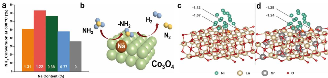
**Fig. 8** (a) Comparison of ammonia decomposition rates *via* Na-doped Co<sub>3</sub>O<sub>4</sub> and Co<sub>3</sub>O<sub>4</sub>-CA. (b) Diagrammatic representation of the catalyst surface ammonia decomposition process.<sup>66</sup> Copyright 2023, Elsevier. Ni/La<sub>2</sub>O<sub>3</sub> (c) and Ni/Sr-La<sub>2</sub>O<sub>3</sub> (d) structural models and Hirshfeld charge of multiple O atoms.<sup>67</sup> Copyright 2020, Elsevier.
