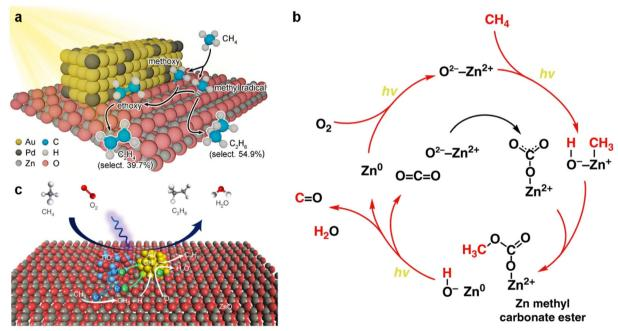
Fig. 5 (a) Scheme of photocatalytic OCM reactions on Pd-modified ZnO-Au. Modified with permission from ref. 72. Copyright (2021) ACS Publications. (b) Scheme of reaction steps in methane photo-oxidation over Zn-HPW/TiO<sub>2</sub>. Modified with permission from ref. 73. Copyright (2019) Springer Nature. (c) Scheme of photocatalytic OCM reactions on an Au nanoparticle (NP) loaded ZnO/TiO<sub>2</sub> hybrid. Modified with permission from ref. 76. Copyright (2021) Springer Nature.
