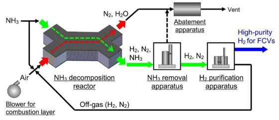
Fig. 4 Scheme of the NH<sub>3</sub>-decomposition fueling station. Modified with permission from ref. 47. Copyright (2023) Elsevier.
