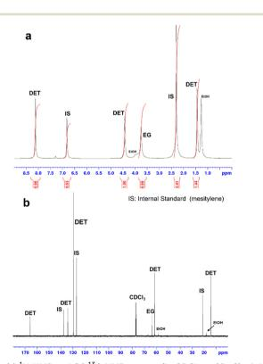
Fig. 1 (a) <sup>1</sup>H NMR and (b) <sup>13</sup>C NMR spectra (in CDCl<sub>3</sub> at 25 °C) of the reaction mixture (at 180 °C for 18 h, run 1) after removal of ethanol. IS (internal standard) = mesitylene.
