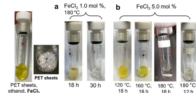
**Fig. 2** Reaction mixture of PET depolymerization with ethanol in the presence of FeCl<sub>3</sub>. Reaction mixture with (a) FeCl<sub>3</sub> (1.0 mol%) at 180 °C (runs 10, 11) and (b) FeCl<sub>3</sub> (5.0 mol%) (runs 1–3, 6).
