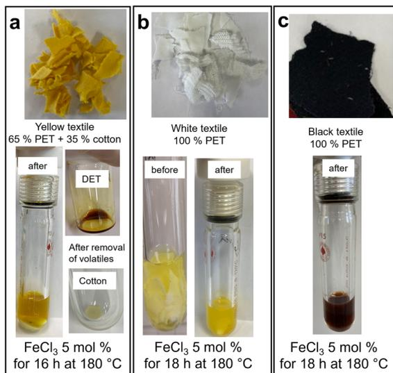
**Fig. 3** Photographs of textile samples (top), and the reactions of textile samples with ethanol in the presence of  $\text{FeCl}_3$  (5.0 mol%) at 180 °C. Photographs of (a) yellow sample (65% PET, 35% cotton) after the reaction, (b) white sample (100% PET), before (left) and after (right) the reaction, (c) black sample after the reaction.
