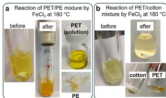
**Fig. 4** Photographs of selective depolymerization of PET from (a) a mixture of PET sheets (by cutting a PET drink bottle) and cotton and (b) PET sheets and polyethylene (PE) with ethanol in the presence of FeCl<sub>3</sub> (5.0 mol%) at 180 °C for 18 h.
