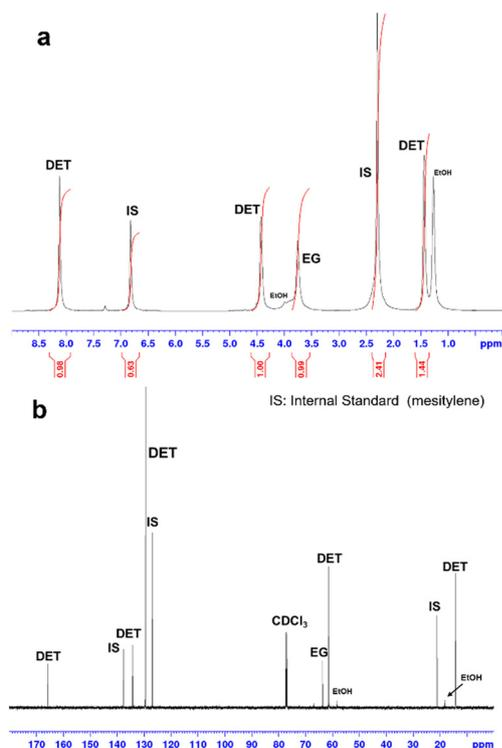
**Fig. 1** (a) <sup>1</sup>H NMR and (b) <sup>13</sup>C NMR spectra (in CDCl<sub>3</sub> at 25 °C) of the reaction mixture (at 180 °C for 18 h, run 1) after removal of ethanol. IS (internal standard) = mesitylene.
