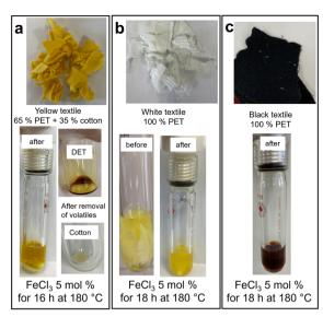
Fig. 3 Photographs of textile samples (top), and the reactions of textile samples with ethanol in the presence of FeCl<sub>3</sub> (5.0 mol%) at 180 °C. Photographs of (a) yellow sample (65% PET, 35% cotton) after the reaction, (b) white sample (100% PET), before (left) and after (right) the reaction, (c) black sample after the reaction.
