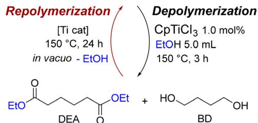
**Scheme 2** Closed-loop chemical recycling (one-pot depolymerization and re-condensation polymerization) of PBA by one-pot depolymerization/re-polycondensation.<sup>42</sup> Reprinted with permission ref. 42. Copyright 2023 by the authors; licensee MDPI.
