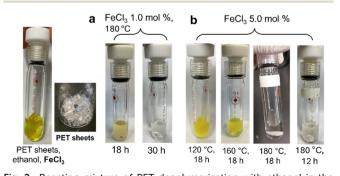
Fig. 2 Reaction mixture of PET depolymerization with ethanol in the presence of FeCl<sub>3</sub>. Reaction mixture with (a) FeCl<sub>3</sub> (1.0 mol%) at 180 °C (runs 10, 11) and (b) FeCl<sub>3</sub> (5.0 mol%) (runs 1-3, 6).
