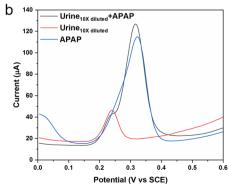
Fig. 6 (a) The selectivity DPV measurement of the CoO-FBC/GCE against interferences of uric acid (UA), ascorbic acid (AA), urea (UREA) and glucose (GLU), all the interference solutions concentration are 200 µM in 0.1 M PBS, and the APAP concentration is 10 µM in 0.1 M PBS; (b) the DPV measurement of the urine sample, where the urine is diluted 10 times in 0.1 M PBS, and the APAP concentration is 100  $\mu$ M in 0.1 M PBS.
