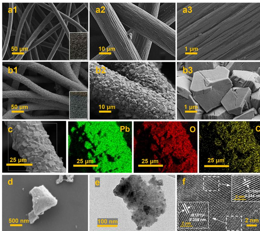
Fig. 2 (a1–a3) SEM images of bare CF substrate (inset: optical photograph); (b1–b3) SEM image of PbO<sub>2</sub>/CF (inset: optical photograph); (c) EDX elemental mapping images of PbO<sub>2</sub>/CF; (d) SEM, (e) TEM, and (f) HRTEM images of the PbO<sub>2</sub> nanocrystals stripped from PbO<sub>2</sub>/CF.
