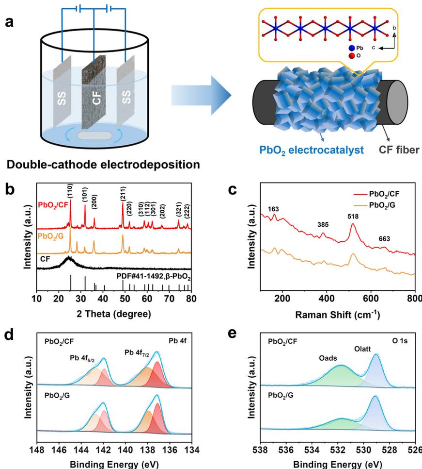
**Fig. 1** (a) Schematic illustration of the double-cathode electrodeposited method for the synthesis of  $\text{PbO}_2/\text{CF}$  and the growth of loaded  $\text{PbO}_2$ ; (b) XRD patterns of  $\text{PbO}_2/\text{CF}$ ,  $\text{PbO}_2/\text{G}$  and CF substrate with the PDF card of  $\beta\text{-PbO}_2$ ; (c) Raman spectra of  $\text{PbO}_2/\text{CF}$  and  $\text{PbO}_2/\text{G}$ ; XPS (d) Pb 4f and (e) O 1s spectra of  $\text{PbO}_2/\text{CF}$  and  $\text{PbO}_2/\text{G}$ .
