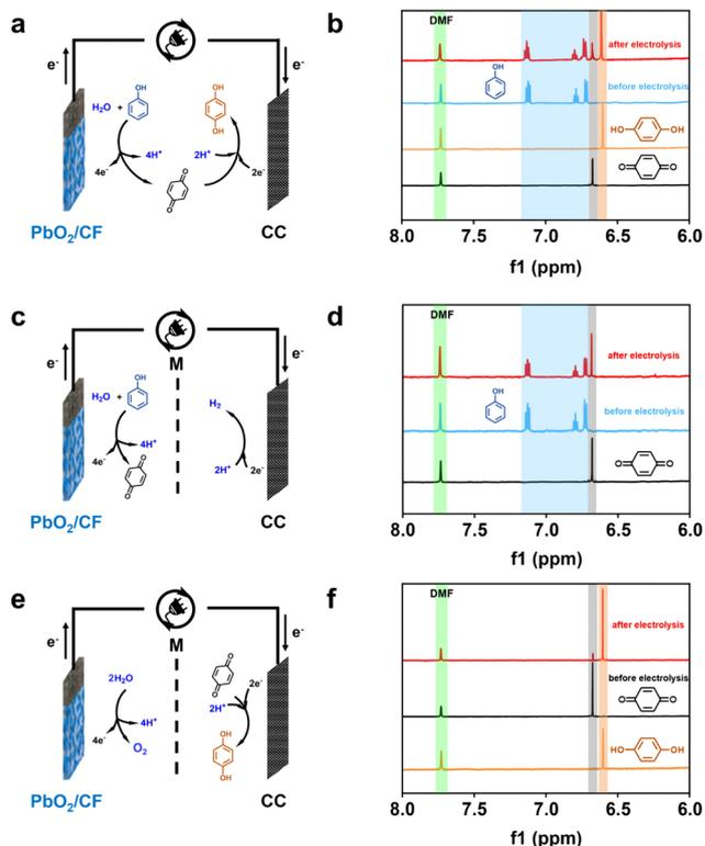
Fig. 4 Reaction pathways in diverse electrolysis configurations and the corresponding  $^1\text{H}$  NMR spectra of substrates and products. (a and b) Membrane-free sequential paired electrosynthesis of 1,4-HQ from phenol; (c and d) membrane-separated phenol oxidation reaction coupling with the HER (e and f) membrane-separated *p*-benzoquinone reduction reaction coupling with the OER.
