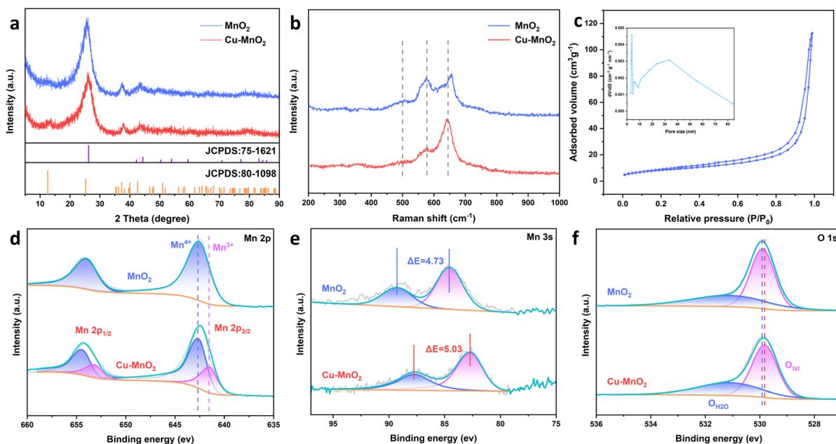
Fig. 3 (a) XRD curves, (b) Raman spectra, (c) N<sub>2</sub> sorption isotherms and pore-size distribution of Cu-MnO<sub>2</sub>. (d) XPS spectra of Mn 2p. (e) XPS spectra of Mn 3s. (f) O 1s XPS spectra of Cu-MnO<sub>2</sub>.
