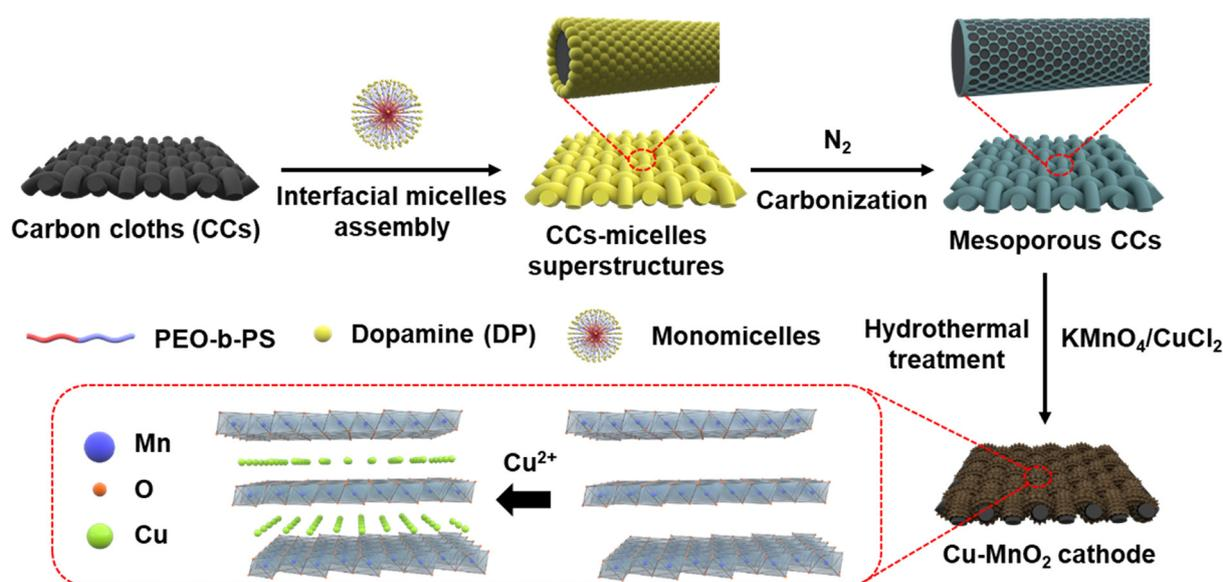
Fig. 1 Synthesis of  $Cu$ - $MnO_2$  (schematic).
