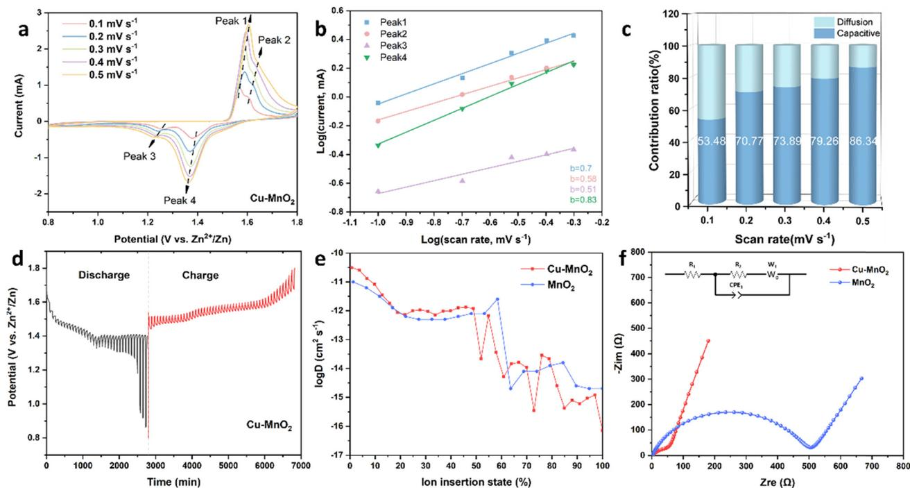
Fig. 5 (a) CV curves of 0.1–0.5 mV s<sup>-1</sup>. (b) Corresponding dependence of log *i* versus log *v* at selected oxidation/reduction states. (c) Capacitive-controlled ratio at various scan rates. (d) GITT curves of Cu-MnO<sub>2</sub>. (e) Diffusion coefficient of Cu-MnO<sub>2</sub> and  $\delta\text{-MnO}_2$ . (f) EIS spectra.
