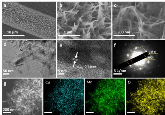
Fig. 2 (a–c) SEM images, (d) TEM image, (e) HRTEM image, (f) SAED pattern, and (g) HAADF-STEM image and corresponding elemental mapping images of Cu-MnO<sub>2</sub>.
