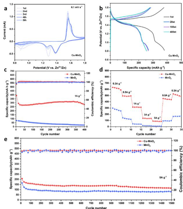
**Fig. 4** (a) CV curves at  $0.1 \text{ mV s}^{-1}$ . (b) GCD curves at  $1.0 \text{ A g}^{-1}$  of Cu-MnO<sub>2</sub>. (c) Cycling performance of Cu-MnO<sub>2</sub> and  $\delta$ -MnO<sub>2</sub> at a current density of  $1.0 \text{ A g}^{-1}$ . (d) Rate performance for Cu-MnO<sub>2</sub> and  $\delta$ -MnO<sub>2</sub>. (e) Long-cycling performance at  $5.0 \text{ A g}^{-1}$ .
