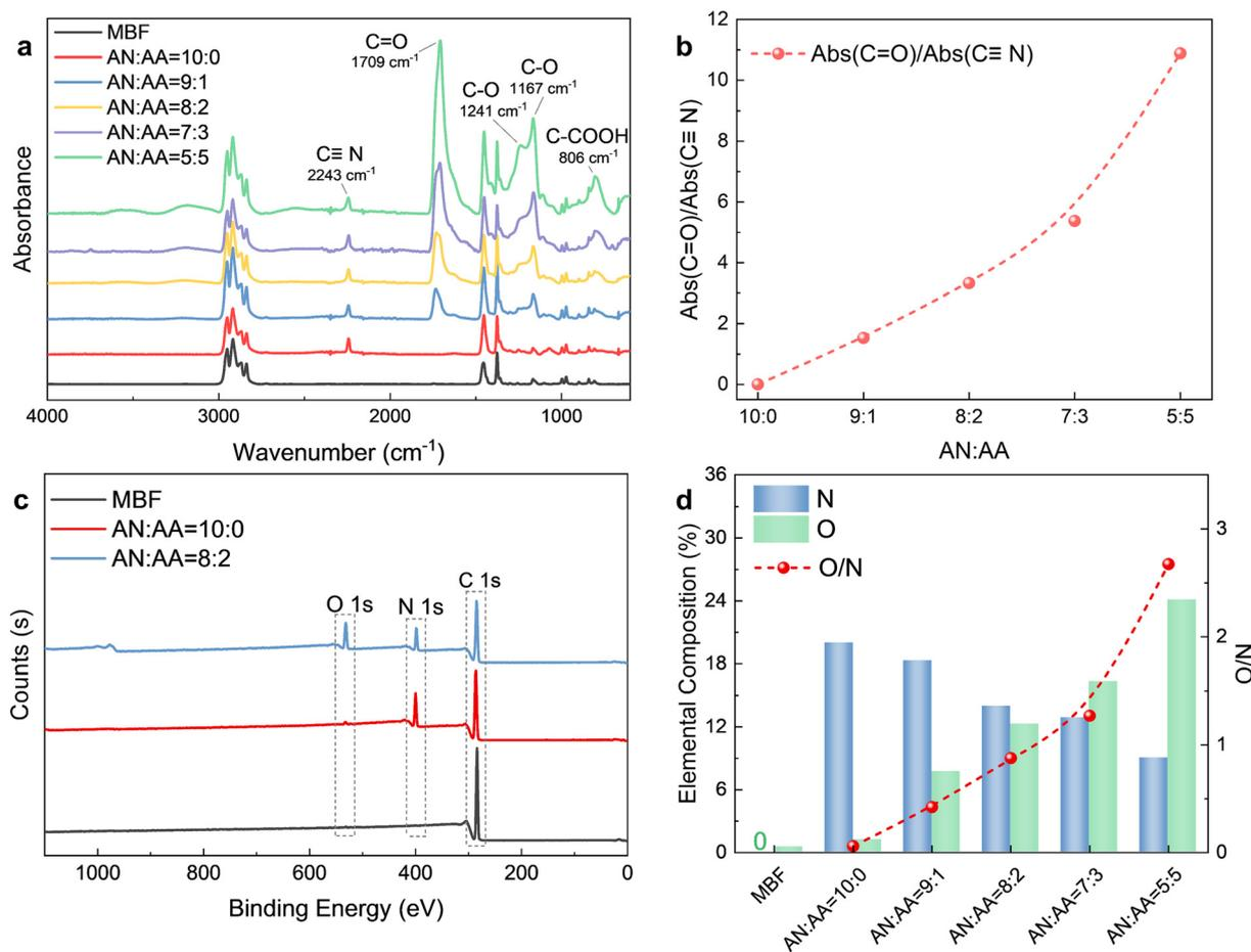
**Fig. 1** (a) The FTIR spectra of the MBF before and after bulk surface photografting with different AN and AA monomer ratios; (b) the ratio of C=O to C≡N absorption peak intensity for different monomer ratios; (c) XPS survey spectra and (d) elemental composition for the MBF before and after photografting.
