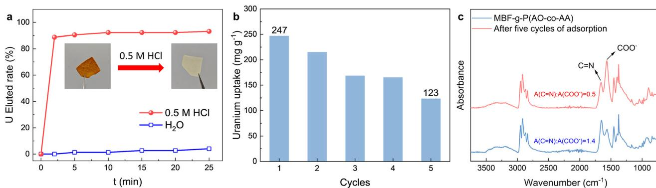
**Fig. 7** (a) Elution efficiency of uranium in 0.5 M HCl and H<sub>2</sub>O; (b) uranium adsorption performance during 5 adsorption-desorption cycles; (c) the FTIR spectra of MBF-g-P(AO-co-AA) initially and after five cycles of adsorption.
