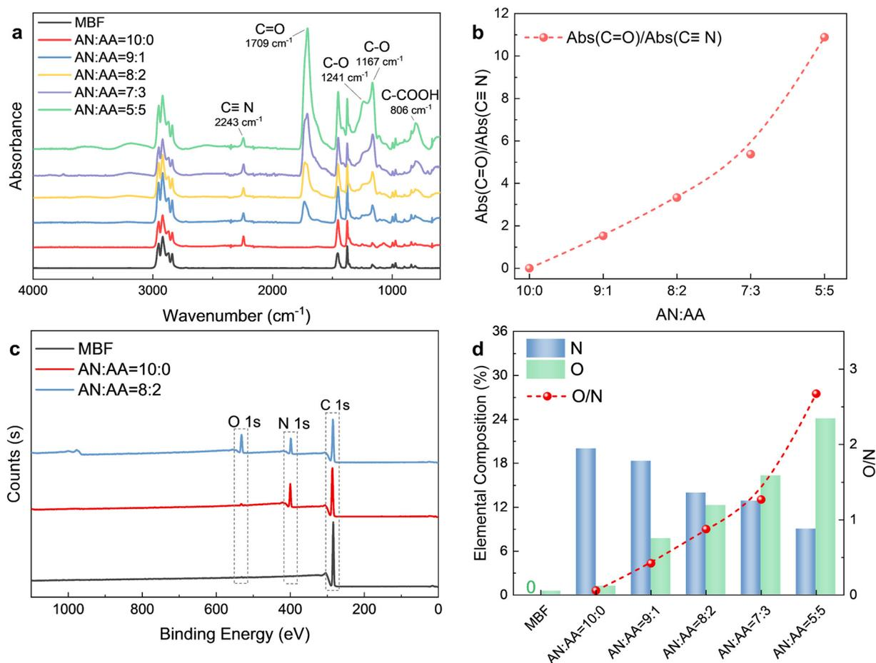
**Fig. 1** (a) The FTIR spectra of the MBF before and after bulk surface photografting with different AN and AA monomer ratios; (b) the ratio of C=O to C≡N absorption peak intensity for different monomer ratios; (c) XPS survey spectra and (d) elemental composition for the MBF before and after photografting.
