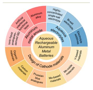
Fig. 2 Modification strategies for aqueous rechargeable Al metal batteries
