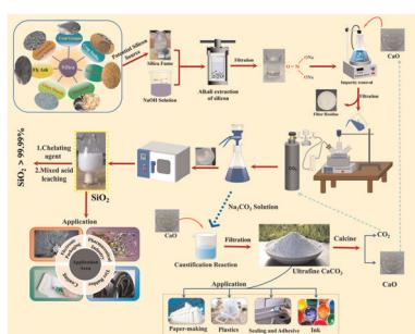
**A green route for producing high-purity nano- $\text{SiO}_2$  from silicon containing waste**
