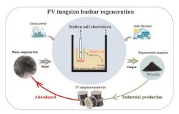
Co-recovery of tungsten and lanthanum from photovoltaic tungsten-based busbars scrap by molten salt electrolysis
