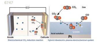
Highly selective, catalyst-free CO<sub>2</sub> reduction in strong acid without alkali cations by a mechanical energy-induced triboelectric plasma-electrolytic system
