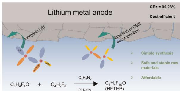
**Rational design of a cost-efficient and eco-friendly fluorinated ether for high-energy and long-lived Li-metal batteries**
