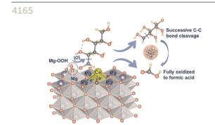
Tailoring the electronic structure and acid-base properties of MgO by Ce doping promotes biomass-derived formic acid production at room temperature
