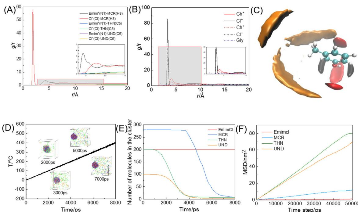
**Fig. 10** RDF between EmimCl and each molecule (A). RDF between ChCl:Gly and MCR (B). SDF of surrounding molecules centered on MCR. Red, black and yellow surfaces represent Emim<sup>+</sup>, Cl<sup>-</sup> and THN, respectively (C). Structural snapshot of simulated flash heating process at different temperatures (D). Number of molecules in cluster at 0.04 bar (E). MSD of the molecules at the interface (F).
