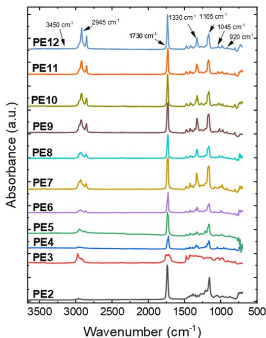
Fig. 6 Synchrotron FT-IR spectra of  $\text{PE}_{n\text{CH}_2\text{s}}$  in the  $3750$ – $750 \text{ cm}^{-1}$  range at  $-40 \text{ }^\circ\text{C}$  after a cooling from the melt at  $20 \text{ }^\circ\text{C min}^{-1}$ . PE3 and PE5 spectra was obtained at RT after an isothermal crystallization.
