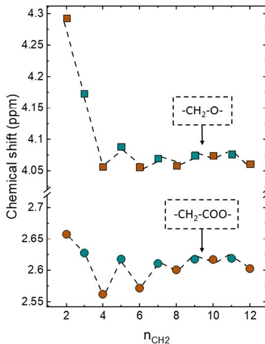
Fig. 2 Chemical shift variation against the  $\text{CH}_2$  number in the chain of the signals attributed to  $-\text{CH}_2-\text{O}-$  (4–4.3 ppm) and  $-\text{CH}_2-\text{COO}-$  (2.5–2.7 ppm). A color code is used to distinguish even-numbered (brown) and odd-numbered (blue) samples.
