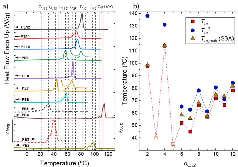
Fig. 13 (a) Final heating after the SSA protocol was applied to the indicated samples. We used the following conditions for the SSA protocol:  $T_{s,\text{ideal}} = 113^\circ\text{C}$ , a fractionation window of  $5^\circ\text{C}$ , and scan rates of  $20^\circ\text{C min}^{-1}$ . (b)  $T_m$ ,  $T_m^0$  and  $T_{m,\text{peak}}$  (SSA) as a function of  $n_{\text{CH}_2}$ .
