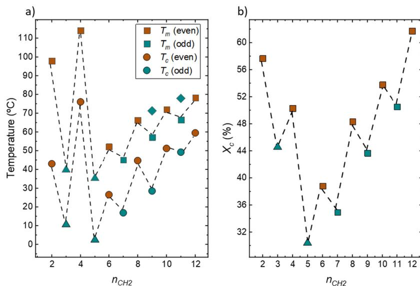
**Fig. 4** (a)  $T_c$  and  $T_m$  as a function of the  $n_{\text{CH}_2}$  in the repeating unit of the  $\text{PE}n_{\text{CH}_2}$ s employed. The triangles represent the data obtained by micro-DSC, while the squares and circles represent the data obtained by DSC. The rhombus symbols indicate the second melting peak in PE9 and PE11. (b)  $X_c$  variation as a function of  $n_{\text{CH}_2}$ . A color code is used to distinguish even-numbered (brown) and odd-numbered (blue) samples.
