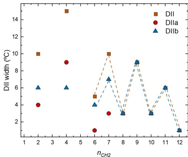
Fig. 12 Memory effect evaluation by taking the *Domain II* variation with chain length ( $n_{\text{CH}_2}$ ).
