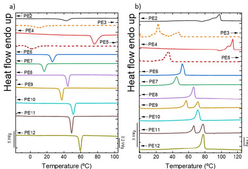
**Fig. 3** Non-isothermal (a) cooling and (b) subsequent heating scans for all the samples. In the case of PE3 and PE5, indicated with dashed lines, they were measured using a Calvet microcalorimeter at  $0.1\text{ °C min}^{-1}$  cooling rate and  $1\text{ °C min}^{-1}$  heating rate, while the rest of the samples were measured by DSC at  $20\text{ °C min}^{-1}$  cooling and heating rate.
