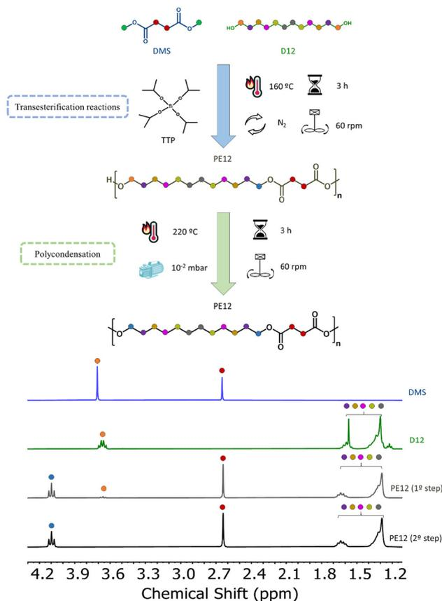
**Fig. 1** Synthetic route for the preparation of PE12. <sup>1</sup>H-NMR spectra of the DMS and D12 monomers and both PE12, before and after the polycondensation step, were included.
