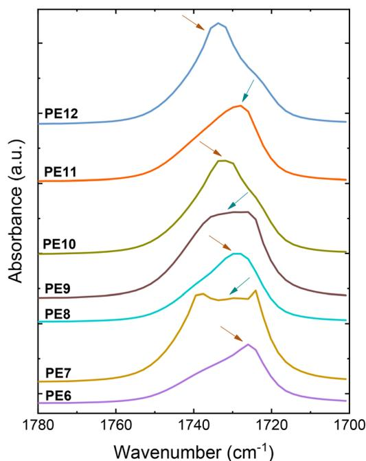
Fig. 7 Comparison of  $n_{\text{CH}_2} > 5$  samples in the carbonyl ( $\text{C}=\text{O}$ ) bands at  $-40 \text{ }^\circ\text{C}$  after a cooling at  $20 \text{ }^\circ\text{C min}^{-1}$ . The arrows indicate the main peaks.
