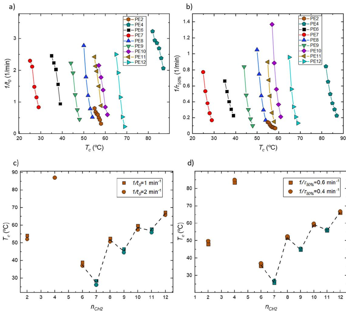
**Fig. 9** (a)  $1/t_0$  vs.  $T_c$  and (b)  $1/\tau_{50\%}$  vs.  $T_c$  obtained after isothermal crystallization. (c)  $T_c$  (at constant  $1/t_0$  value) and (d)  $T_c$  (at constant  $1/\tau_{50\%}$  value) against  $n_{\text{CH}_2}$ . A color code is used to distinguish even-numbered (brown) and odd-numbered (blue) samples.
