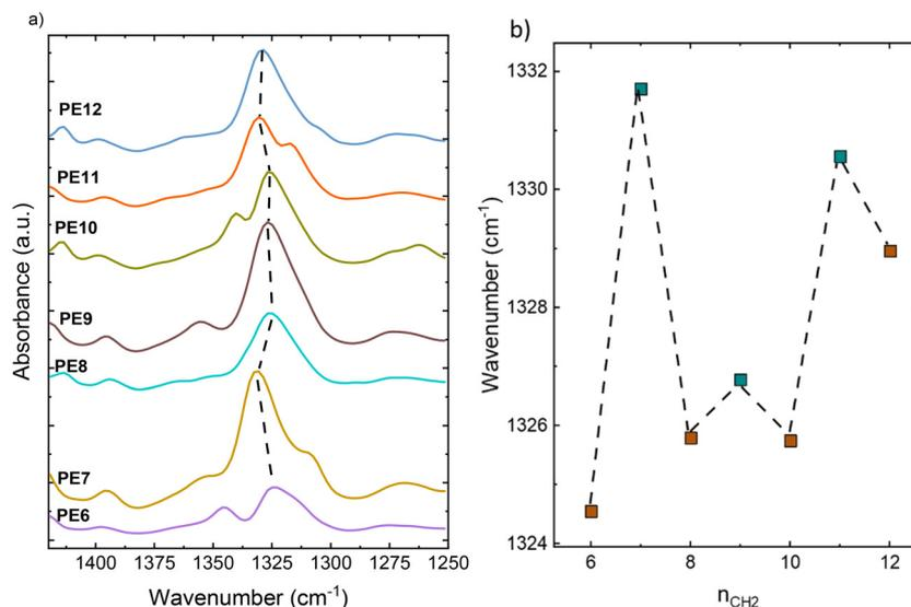
**Fig. 8** (a) Comparison of  $n_{\text{CH}_2} > 5$  samples in symmetric deformation of the  $-\text{CH}_2-$  group bands at  $-40^\circ\text{C}$  after a cooling at  $20^\circ\text{C min}^{-1}$ . (b) Symmetric deformation  $-\text{CH}_2-$  peak variation as a function of  $n_{\text{CH}_2}$ . A color code is used to distinguish even-numbered (brown) and odd-numbered (blue) samples.
