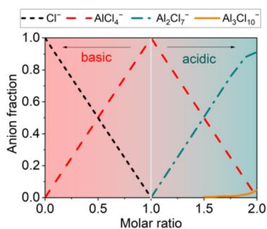
**Fig. 12** The anion speciation diagram of  $\text{AlCl}_3/[\text{EMIm}]\text{Cl}$  at room temperature, illustrating the electrolyte compositions at  $0 < r < 2$ . Adapted from Palacin, M. R. *et al.*, *J. Phys.: Energy*.<sup>107</sup> Licensed under CC BY 4.0. ©2024 IOP Publishing.
