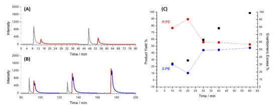
Fig. 3 Chromatograms of the fractions collected after (A) 10 and 20 minutes and (B) 30, 40 and 60 minutes from the  $\delta^+$  extremity of the Ppy tube with citronellol-based NCIL by applying a constant electric field of 2.8 V cm $^{-1}$ . The red and blue colors stand for R- and S-PE, respectively, while the grey peaks are related to AP. In (C) the corresponding enantiomeric excess (in red or blue) and apparent product yield (in black) as a function of the time of electrolysis are reported.
