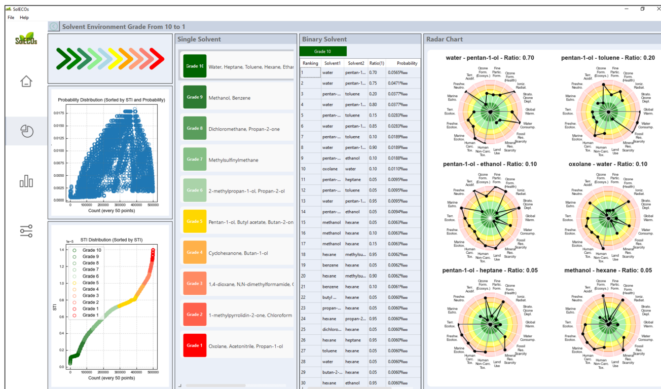
Fig. 7 SoIECOs interface – APAP case study screenshot. The interface displays the classification of single and binary solvents by sustainability grade, including solvent identity, composition, and probability. The right panel shows radar plots of the top six binary solvent combinations with the highest probabilities, where each axis represents one of 18 midpoint indicators normalized to a 0–1 scale.
