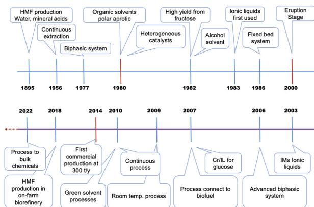
Fig. 3 The significant milestones of HMF synthesis since its discovery in 1895. Reproduced from ref. 5 with permission from the RSC,<sup>5</sup> copyright 2014.
