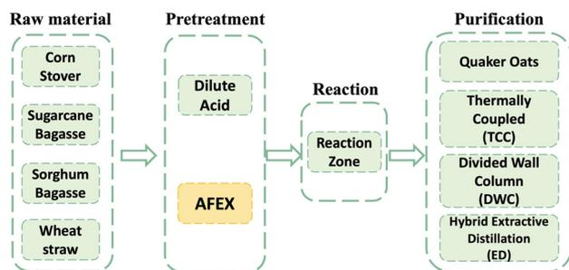
Fig. 12 Diagram illustrating the different possible scenarios studied by Contreras-Zarazúa *et al.* Adapted from ref. 78 with permission from Elsevier,<sup>78</sup> copyright 2022.
