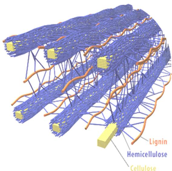
**Fig. 14** Spatial arrangement of cellulose, hemicellulose and lignin in the cell walls of lignocellulosic biomass. Adapted from ref. 161 with permission from the U.S. Department of Energy Genomic Science program,<sup>161</sup> copyright 2011.
