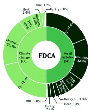
Fig. 8 Sunburst chart for the environmental impact of biomass-derived FDCA. Adapted from ref. 57 with permission from the RSC,<sup>57</sup> copyright 2020.
