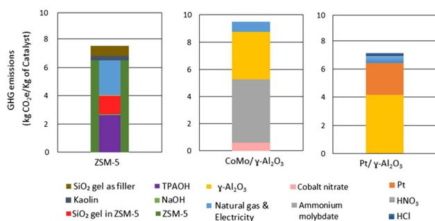
**Fig. 13** Cradle-to-gate GHGs for the synthesis of ZSM-5, CoMo/ $\gamma$ -Al<sub>2</sub>O<sub>3</sub>, and Pt/ $\gamma$ -Al<sub>2</sub>O<sub>3</sub>. Adapted from ref. 147 with permission from Elsevier,<sup>147</sup> copyright 2017.
