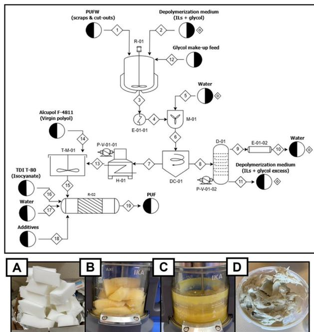
**Fig. 6** Process flow diagram described in the SI (see Tables S3 and S4) (top). PUFW cut-outs before starting the process (A); PUFW homogenized with the IL mixture and EG after 30 minutes (B); overall reaction medium after 4 hours (C); dry recycled polyol (D) (bottom). Conditions: 343 g of [Bmim][Cl] (1.96 mol), 147 g of [Bmim][OAc] (0.74 mol), 50 g of EG (0.81 mol) and 100 g of PUFW, 98 °C, 4 h and 100 rpm.
