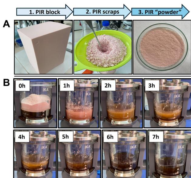
**Fig. 5** (A) Mechanical pretreatment of PIR; (B) scale-up PIR depolymerization process after each hour of reaction, until reaching a homogeneous overall medium. Conditions: 400 g of [Bmim][Cl] (2.29 mol), 300 g of [Bmim][OAc] (1.51 mol), 100 g of ethylene glycol (1.61 mol) and 50 g of PIR, 115 °C, 7 h, 100 rpm.
