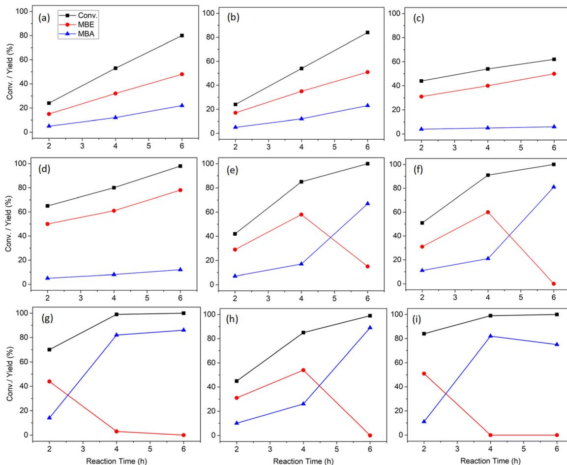
**Fig. 8** Catalytic conversion with product distribution for different reaction times at 30 °C for (a) 10Ni/Ti-M\_300, (b) 10Ni/Ti-M\_400, (c) 10Ni/Ti-M\_500, (d) 10Ni/Ti-A\_300, (e) 10Ni/Ti-A\_400, (f) 10Ni/Ti-A\_500, (g) 10Ni/Ti-R\_300, (h) 10Ni/Ti-R\_400, and (i) 10Ni/Ti-R\_500 catalysts. Reaction conditions: MBY – 1 g, H<sub>2</sub>O – 40 g, catalyst – 100 mg, temp. – 30 °C, time – 6 h, H<sub>2</sub> – 10 bar (at 30 °C), and RPM – 900.
