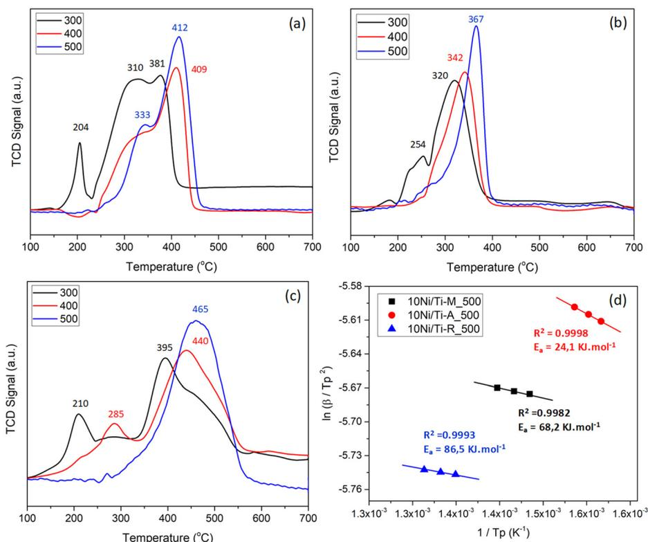
**Fig. 4** H<sub>2</sub>-TPR profiles of (a) 10Ni/Ti-M, (b) 10Ni/Ti-A, and (c) 10Ni/Ti-R catalysts calcined at 300, 400 and 500 °C and (d) Kissinger plot of the three 10%Ni–titania catalysts.
