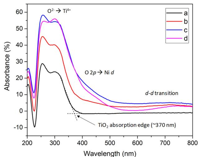
Fig. 3 DRUV-Vis profiles of the calcined nickel catalyst on different titania: (a) Ti-M, (b) 10Ni/Ti-M\_500, (c) 10Ni/Ti-A\_500 and (d) 10Ni/Ti-R\_500.
