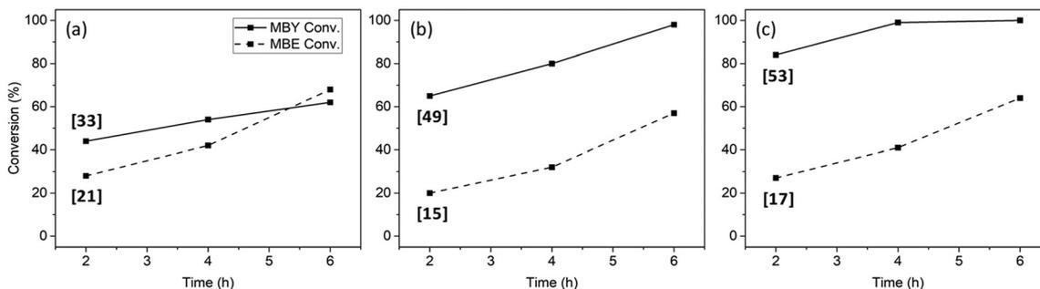
**Fig. 9** Conversion of MBY and MBE for (a) 10Ni/Ti-M\_500, (b) 10Ni/Ti-A\_500, and (c) 10Ni/Ti-R\_500 catalysts. The numbers in square brackets represent TON at 2 h. Reaction conditions: reactant – 1 g, H<sub>2</sub>O – 40 g, catalyst – 100 mg, temp. – 30 °C, time – 2–6 h, H<sub>2</sub> – 10 bar (at 30 °C), and RPM – 900.
