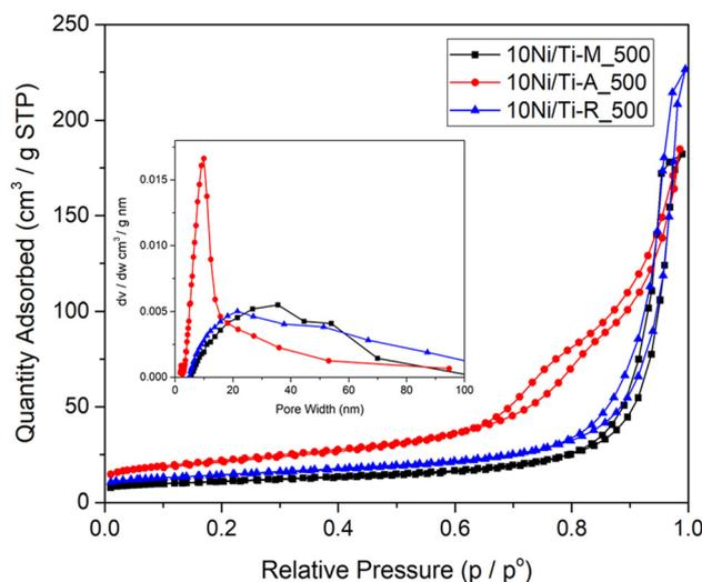
Fig. 1 N<sub>2</sub> adsorption–desorption isotherms (inset: pore size distribution) of nickel-supported catalysts prepared by wet impregnation.
