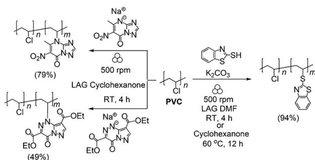
**Scheme 16** Functionalization of waste PVC by grafting azole-containing drugs under LAG ball milling conditions.<sup>103</sup>
