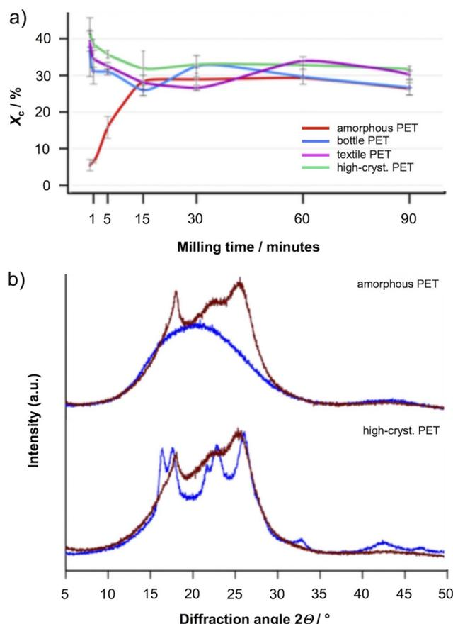
**Fig. 6** (a) The effect of milling on percent crystallinity of different types of PET at 30 Hz frequency. (b) PXRD analysis of amorphous and high-crystallinity PET samples before (blue) and after (brown) 90 minutes of milling at 30 Hz. Adapted with permission from A. Zaker and K. Auclair, Impact of Ball Milling on the Microstructure of Polyethylene Terephthalate, *ChemSusChem*, 2025, **18**, e202401506.<sup>33</sup>
