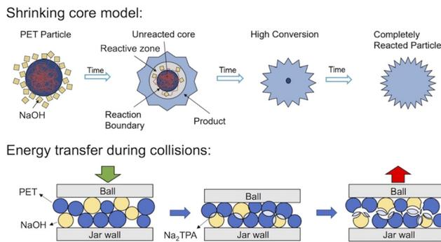
**Fig. 4** Shrinking core model proposed for the alkaline PET depolymerization under ball milling conditions. Reprinted with permission from A. W. Tricker, A. A. Osibo, Y. Chang, J. X. Kang, A. Ganesan, E. Anglou, F. Boukouvala, S. Nair, C. W. Jones and C. Sievers, Stages and Kinetics of Mechanochemical Depolymerization of Poly(ethylene terephthalate) with Sodium Hydroxide, *ACS Sustainable Chem. Eng.*, 2022, **10**, 11338–11347. Copyright 2022, American Chemical Society.<sup>30</sup>
