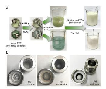
Fig. 1 (a) Schematic diagram of TPA isolation from waste PET. (b) Rheology changes during ball milling PET and NaOH under solvent-free or LAG conditions.<sup>29</sup>
