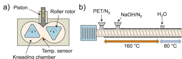
**Fig. 22** (a) Schematic diagram of a laboratory kneader used by Scholl to depolymerize PET with NaOH on a 30 gram scale.<sup>127</sup> (b) Scheme of continuous alkaline depolymerization of PET by reactive extrusion.<sup>129</sup>
