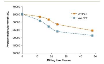
Fig. 5 The effect of moisture on PET polymer chain scission during ball milling of dry and wet samples.  $M_{\rm w}$  values were measured in a phenol: o-cresol (1:1) mixture by solution viscometry. 35
