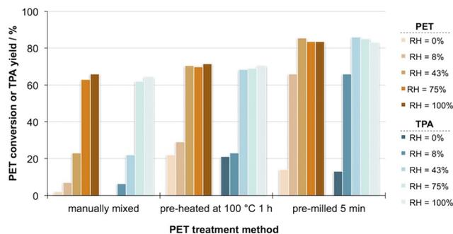
**Fig. 2** PET conversion and TPA yield during aging at different humidity levels for 3 days at 25 °C as a function of the PET treatment method.<sup>29</sup>
