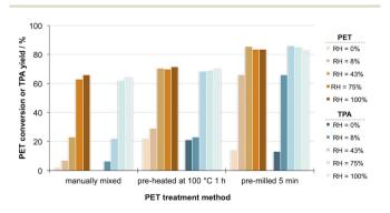
Fig. 2 PET conversion and TPA yield during aging at different humidity levels for 3 days at 25 °C as a function of the PET treatment method.<sup>29</sup>
