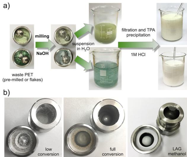
**Fig. 1** (a) Schematic diagram of TPA isolation from waste PET. (b) Rheology changes during ball milling PET and NaOH under solvent-free or LAG conditions.<sup>29</sup>
