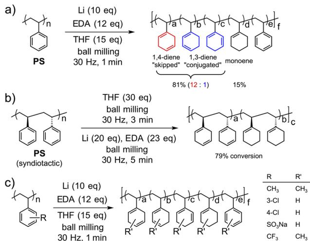
**Scheme 8** (a) The mechanochemical Birch reduction of polystyrene using the Li/EDA system. (b) The Birch reduction of syndiotactic polystyrene. (c) Substrate scope of the Birch reduction by ball milling.<sup>81</sup>
