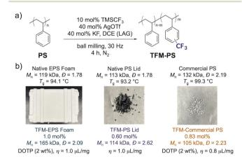
Fig. 14 (a) Electrophilic trifluoromethylation strategy for grafting polystyrene by ball milling. (b) Examples of post-consumer and commercial polystyrene samples functionalized with  $CF_3$  groups under LAG conditions and in the presence of DOTP plasticizer. Adapted with permission from M. E. Skala, S. M. Zeitler and M. R. Golder, Liquid-assisted grinding enables a direct mechanochemical functionalization of polystyrene waste, *Chem. Sci.*, 2024, 15, 10900–10907.<sup>78</sup>
