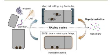
Fig. 17 Schematic representation of the RAging technique for the hydrolysis of biopolymers and synthetic polymers.<sup>118</sup>
