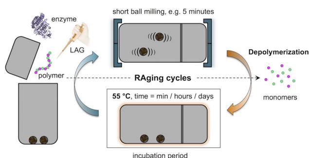
**Fig. 17** Schematic representation of the RAgging technique for the hydrolysis of biopolymers and synthetic polymers.<sup>118</sup>
