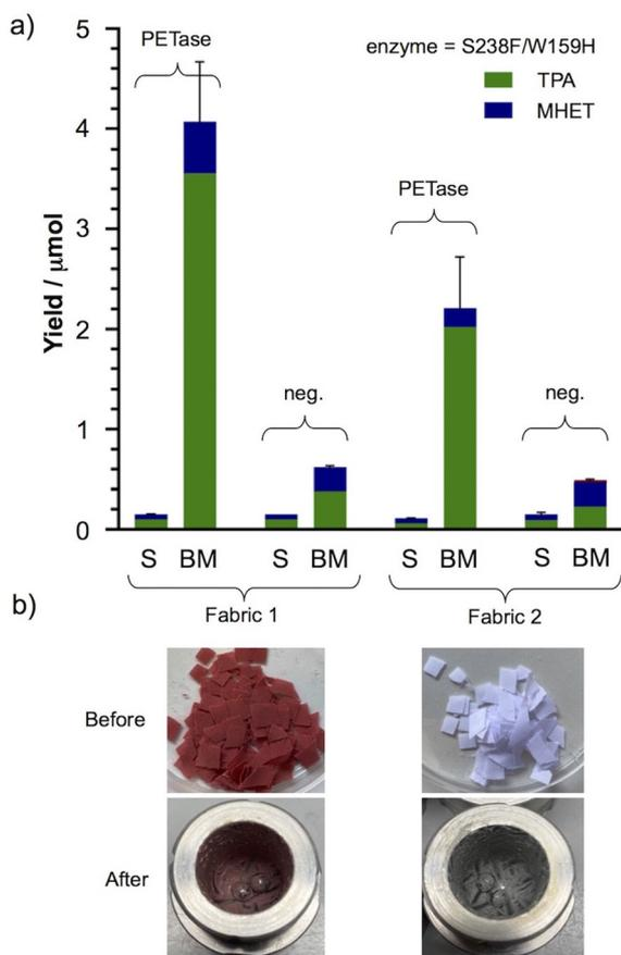
**Fig. 19** (a) Enzymatic depolymerization of two samples of PET fabric in solution (S) and under ball milling (BM). (b) PET fabric samples before and after mechanoenzymatic hydrolysis. Adapted with permission from E. Ambrose-Dempster, L. Leipold, D. Dobrijevic, M. Bawn, E. M. Carter, G. Stojanovski, T. D. Sheppard, J. W. E. Jeffries, J. M. Ward and H. C. Hailes, Mechanoenzymatic reactions for the hydrolysis of PET, *RSC Adv.*, 2023, **13**, 9954–9962.<sup>120</sup>
