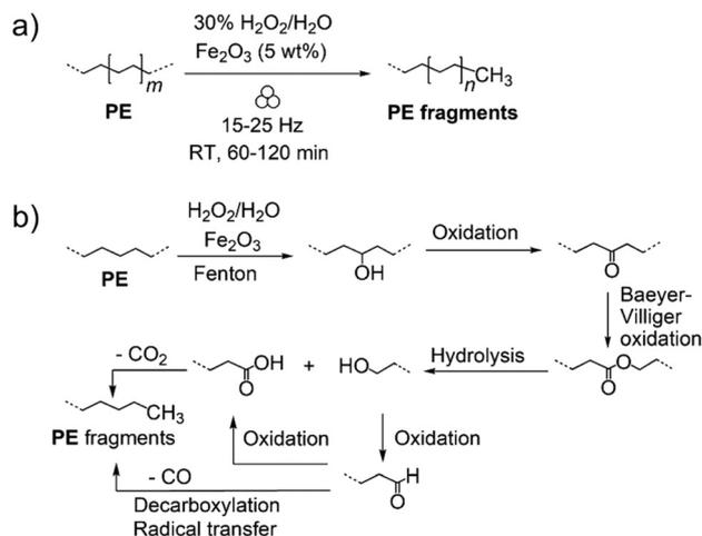
**Scheme 4** (a) Depolymerization of MDPE by the Fenton process under ball milling conditions. (b) Proposed mechanism for the mechanocatalytic Fenton-type depolymerization of MDPE by ball milling.<sup>64</sup>
