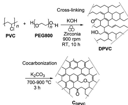
**Scheme 15** Mechanochemical upcycling of waste PVC via KOH/PEG-800 promoted dechlorination and cocarbonization with  $\text{K}_2\text{CO}_3$  at high temperatures.<sup>102</sup>
