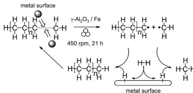
**Scheme 5** Mechanochemical gasification of the PE and PET substrates with hydrogen gas in the presence of  $\gamma\text{-Al}_2\text{O}_3/\text{Fe}$  catalysts. The reaction proceeds by a radical mechanism.<sup>65</sup>
