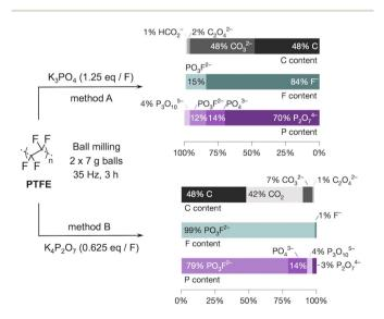
Fig. 15 The effect of K<sub>3</sub>PO<sub>4</sub> and K<sub>4</sub>P<sub>2</sub>O<sub>7</sub> salts on the distribution of carbon, fluorine and phosphorus in the product after ball milling PTFE at 35 Hz for 3 hours. Adapted with permission from L. Yang, Z. Chen, C. A. Goult, T. Schlatzer, R. S. Paton and V. Gouverneur, Phosphateenabled mechanochemical PFAS destruction for fluoride reuse, Nature, 2025, **640**, 100-106. 113
