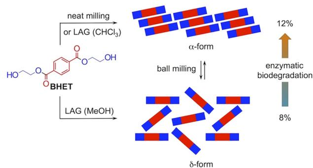
**Fig. 20** Two stable polymorphs of BHET form selectively and interconvert under neat or LAG ball milling conditions. The thermodynamically more stable  $\alpha$ -form is enzymatically hydrolyzed at a faster rate than the  $\delta$ -form.<sup>122</sup>
