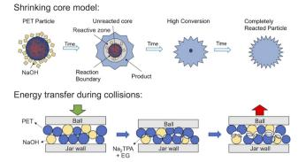
Fig. 4 Shrinking core model proposed for the alkaline PET depolymerization under ball milling conditions. Reprinted with permission from A. W. Tricker, A. A. Osibo, Y. Chang, J. X. Kang, A. Ganesan, E. Anglou, F. Boukouvala, S. Nair, C. W. Jones and C. Sievers, Stages and Kinetics of Mechanochemical Depolymerization of Poly(ethylene terephthalate) with Sodium Hydroxide, ACS Sustainable Chem. Eng., 2022, 10, 11338-11347. Copyright 2022, American Chemical Society.
