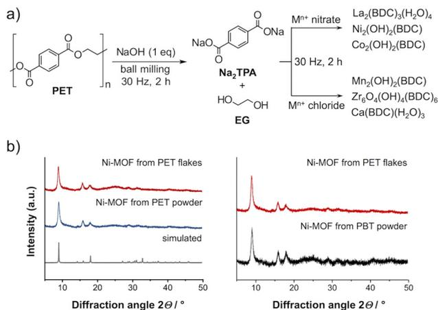
**Fig. 9** (a) Mechanochemical upcycling of waste PET to MOFs. (b) PXRD patterns of the Ni-MOF synthesized from the PET flakes and powder (left), and comparison with the sample prepared from PBT as a source of 1,4-dicarboxylate ligand.<sup>40</sup>
