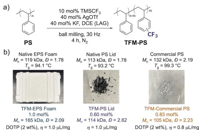
**Fig. 14** (a) Electrophilic trifluoromethylation strategy for grafting polystyrene by ball milling. (b) Examples of post-consumer and commercial polystyrene samples functionalized with CF<sub>3</sub> groups under LAG conditions and in the presence of DOTP plasticizer. Adapted with permission from M. E. Skala, S. M. Zeitzer and M. R. Golder, Liquid-assisted grinding enables a direct mechanochemical functionalization of polystyrene waste, *Chem. Sci.*, 2024, **15**, 10900–10907.<sup>78</sup>
