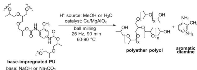
**Scheme 3** Ball milling promoted degradation of a base-impregnated polyurethane in the presence of a  $\text{Cu}/\text{MgAlO}_x$  catalyst at elevated temperatures.<sup>50</sup>
