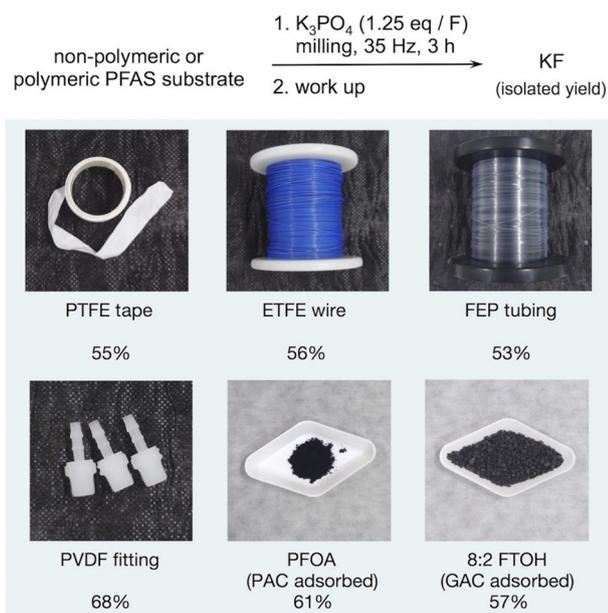
**Fig. 16** Several examples of successful degradation of different commercial PFAS compounds by ball milling in the presence of  $K_3PO_4$  salt (method A) after 3 hours. Adapted with permission from L. Yang, Z. Chen, C. A. Goult, T. Schlatter, R. S. Paton and V. Gouverneur, Phosphate-enabled mechanochemical PFAS destruction for fluoride reuse, *Nature*, 2025, **640**, 100–106.<sup>113</sup>
