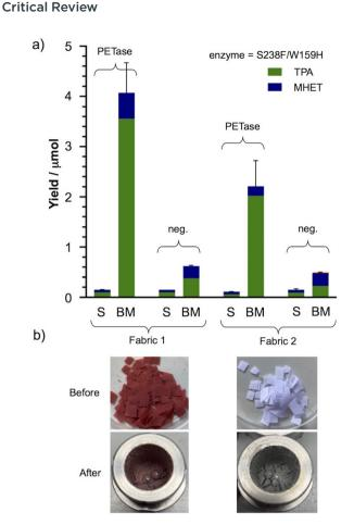
Fig. 19 (a) Enzymatic depolymerization of two samples of PET fabric in solution (S) and under ball milling (BM). (b) PET fabric samples before and after mechanoenzymatic hydrolysis. Adapted with permission from E. Ambrose-Dempster, L. Leipold, D. Dobrijevic, M. Bawn, E. M. Carter, G. Stojanovski, T. D. Sheppard, J. W. E. Jeffries, J. M. Ward and H. C. Hailes, Mechanoenzymatic reactions for the hydrolysis of PET, RSC Adv., 2023, 13, 9954-9962.120
