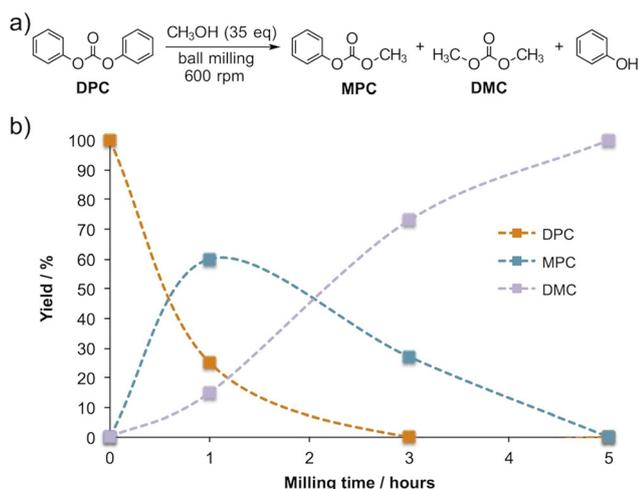
Fig. 8 (a) Mechanochemical methanolysis of diphenyl carbonate (DPC). (b) Concentration profiles during methanolysis of DPC at 600 rpm on a 1 mmol scale.<sup>39</sup>
