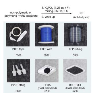
Fig. 16 Several examples of successful degradation of different commercial PFAS compounds by ball milling in the presence of  $\rm K_3PO_4$  salt (method A) after 3 hours. Adapted with permission from L. Yang, Z. Chen, C. A. Goult, T. Schlatzer, R. S. Paton and V. Gouverneur, Phosphate-enabled mechanochemical PFAS destruction for fluoride reuse, *Nature*, 2025, **640**, 100–106.  $^{113}$
