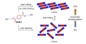
Fig. 20 Two stable polymorphs of BHET form selectively and interconvert under neat or LAG ball milling conditions. The thermodynamically more stable  $\alpha$ -form is enzymatically hydrolyzed at a faster rate than the  $\delta$ -form. 122
