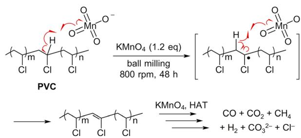
**Scheme 13** Proposed mechanism for the potassium permanganate-promoted oxidation of waste PVC and its transformation to gaseous products.<sup>100</sup>
