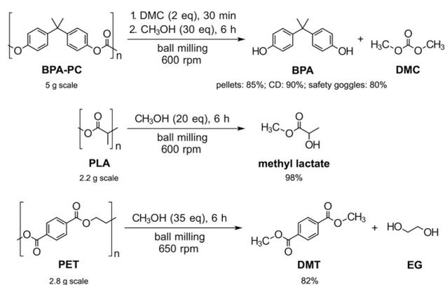
**Scheme 2** Direct methanolysis of polycarbonate BPA-PC and polyesters PLA and PET.<sup>39</sup>
