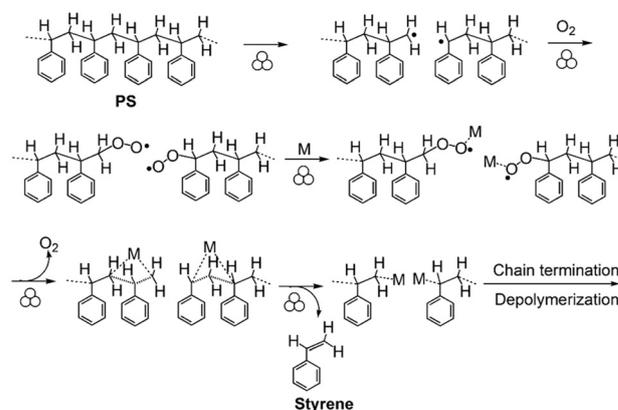
**Scheme 7** Proposed mechanism of ball milling-promoted depolymerization of polystyrene.<sup>74</sup>
