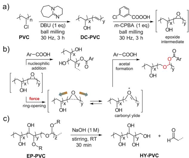
**Scheme 14** (a) A mechanochemical PVC dechlorination/epoxidation sequence. (b) The epoxide intermediate undergoes simultaneous nucleophilic addition and force-induced ring-opening reactions with the formation of acetals. (c) Epoxidized product EP-PVC is hydrolyzed in a NaOH solution with the generation of water-soluble low-molecular-weight non-toxic products.<sup>101</sup>
