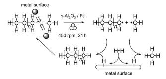
Scheme 5 Mechanochemical gasification of the PE and PET substrates with hydrogen gas in the presence of  $\gamma$ -Al<sub>2</sub>O<sub>3</sub>/Fe catalysts. The reaction proceeds by a radical mechanism.65
