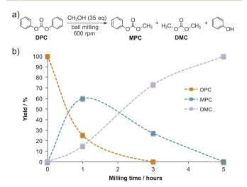
**Fig. 8** (a) Mechanochemical methanolysis of diphenyl carbonate (DPC). (b) Concentration profiles during methanolysis of DPC at 600 rpm on a 1 mmol scale.<sup>39</sup>
