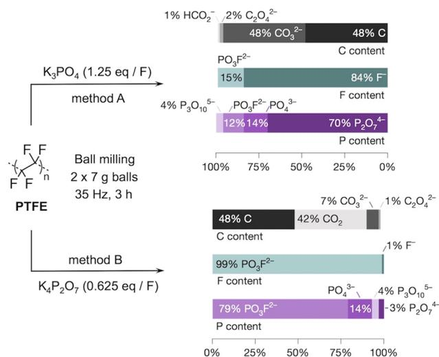
**Fig. 15** The effect of  $\text{K}_3\text{PO}_4$  and  $\text{K}_4\text{P}_2\text{O}_7$  salts on the distribution of carbon, fluorine and phosphorus in the product after ball milling PTFE at 35 Hz for 3 hours. Adapted with permission from L. Yang, Z. Chen, C. A. Gault, T. Schlätzer, R. S. Paton and V. Gouverneur, Phosphate-enabled mechanochemical PFAS destruction for fluoride reuse, *Nature*, 2025, **640**, 100–106.<sup>113</sup>
