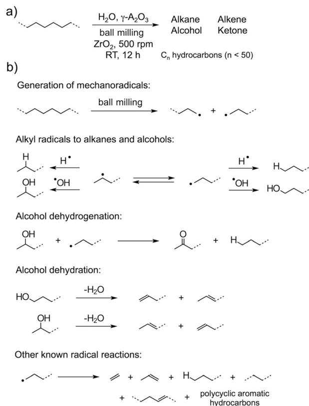
**Scheme 6** (a) Mechanochemical degradation of PE by water activation in the presence of  $\gamma\text{-Al}_2\text{O}_3$  dispersants. (b) Proposed reaction mechanism involves the generation of alkyl radicals by ball milling and subsequent homolytic water splitting to produce alkanes, alcohols, alkenes and ketones.<sup>66</sup>
