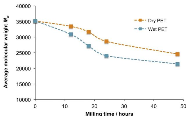
**Fig. 5** The effect of moisture on PET polymer chain scission during ball milling of dry and wet samples.  $M_w$  values were measured in a phenol:*o*-cresol (1:1) mixture by solution viscometry.<sup>35</sup>
