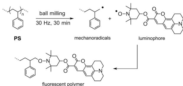
**Scheme 10** Ball milling functionalization of PS with a luminophore molecule enabled by mechanochemically generated macroradicals.<sup>84</sup>
