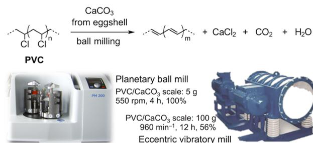
**Fig. 24** Upcycling of waste PVC and biowaste eggshells as a source of CaCO<sub>3</sub> for mechanochemical dechlorination on a laboratory and semi-industrial scale reported by Baláz *et al.*<sup>132</sup>
