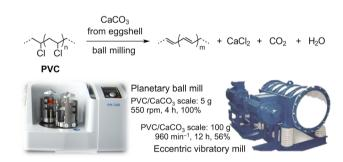
Fig. 24 Upcycling of waste PVC and biowaste eggshells as a source of  $CaCO_3$  for mechanochemical dechlorination on a laboratory and semi-industrial scale reported by Baláž et al. 132
