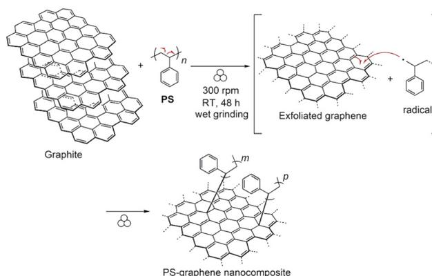
**Scheme 9** Mechanochemical grafting of polystyrene with graphene by wet ball milling.<sup>82</sup>
