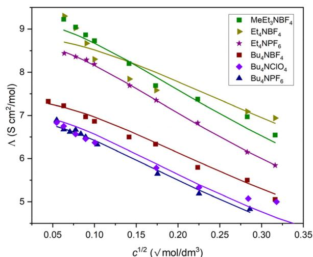
**Fig. 1** Molar conductivity value of tetrabutylammonium salts vs. square root of the concentration in DLG at 298.15 K in the range of 0.002 M to 0.2 M; symbols denote the experimental data, lines denote the LWPT calculations.
