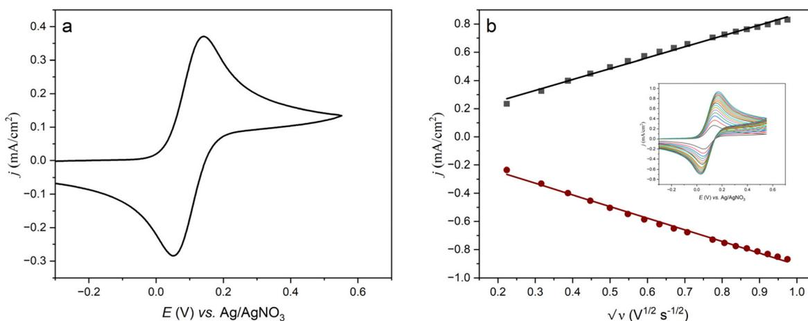
Fig. 7 (a) Cyclic voltammogram of ferrocene ( $5\text{ mM}$ ) at a glassy carbon electrode in DLG ( $0.15\text{ M}$  of  $\text{Bu}_4\text{NBF}_4$ ) at  $298.15\text{ K}$ , Pt as a counter electrode, scan rate  $0.1\text{ V s}^{-1}$ , Ru compensated 90% (b) plot of peak current vs. scan rate square root of the ferrocene in DLG at  $298.15\text{ K}$ .
