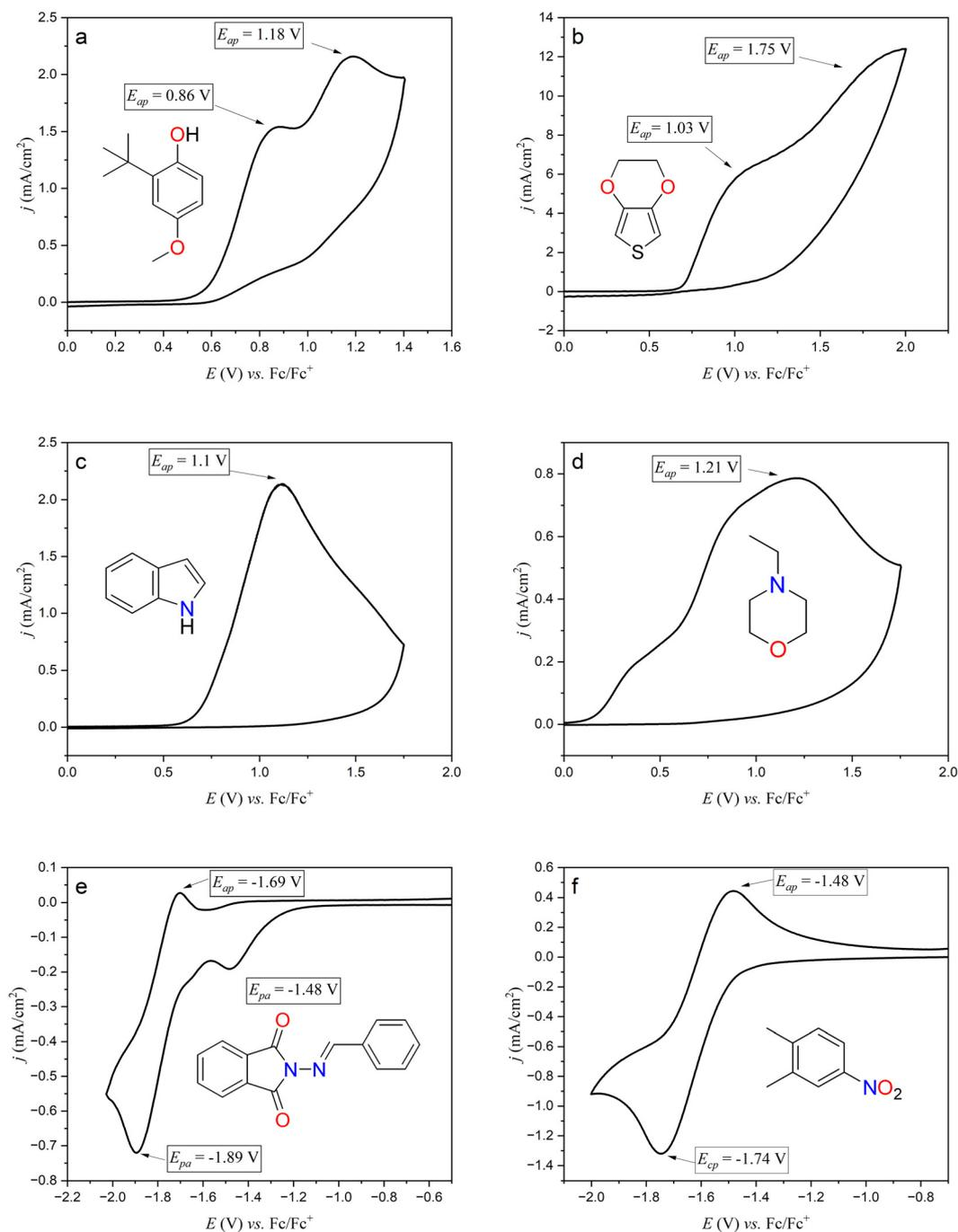
**Fig. 11** Cyclic voltammograms of organic compounds (0.01 M) in DLG at glassy carbon electrode. (a) 3-*tert*-butyl-4-hydroxyanisole, (b) 3,4-ethylenedioxythiophene, (c) indole, (d) 4-ethylmorpholine, (e) *N*-(aminobenzylidene)-phthalimide, (f) 3,4-dimethylnitrobenzene.
