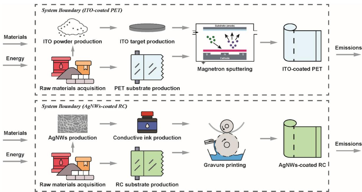
**Fig. 1** System boundary of TCEs. ITO-coated PET films include ITO target (produced from ITO powder), PET substrate, and magnetron sputtering. AgNWs-coated RC films comprise AgNWs-based ink, RC substrate, and gravure printing.
