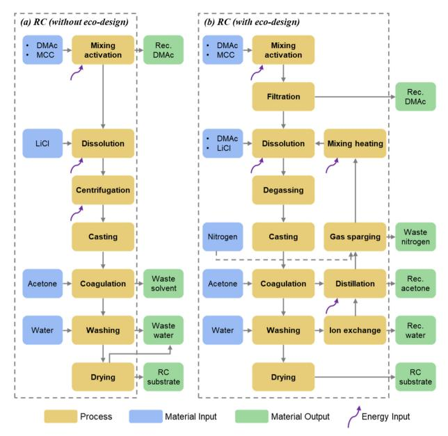
Fig. 3 Process flow chart of RC substrate production using (a) the current synthesis method and (b) eco-design considerations based on various GC Principles. "Rec." denotes recycled.
