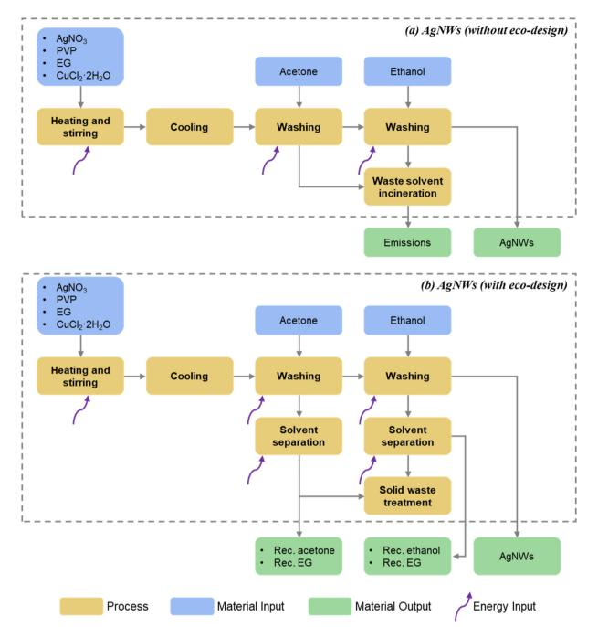
Fig. 2 Process flow chart of AgNWs production using (a) the current polyol method and (b) eco-design considerations based on various GC Principles. "Rec." denotes recycled.
