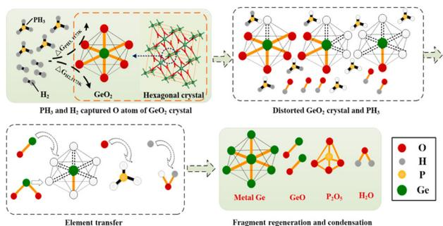
Fig. 5 Reaction mechanism of the vacuum phosphate reduction of  $\text{GeO}_2$  (adapted from ref. 117 with permission from the American Chemical Society, *ACS Sustain. Chem. Eng.*, 2019, 7(2), 2176–2186, Copyright 2018).
