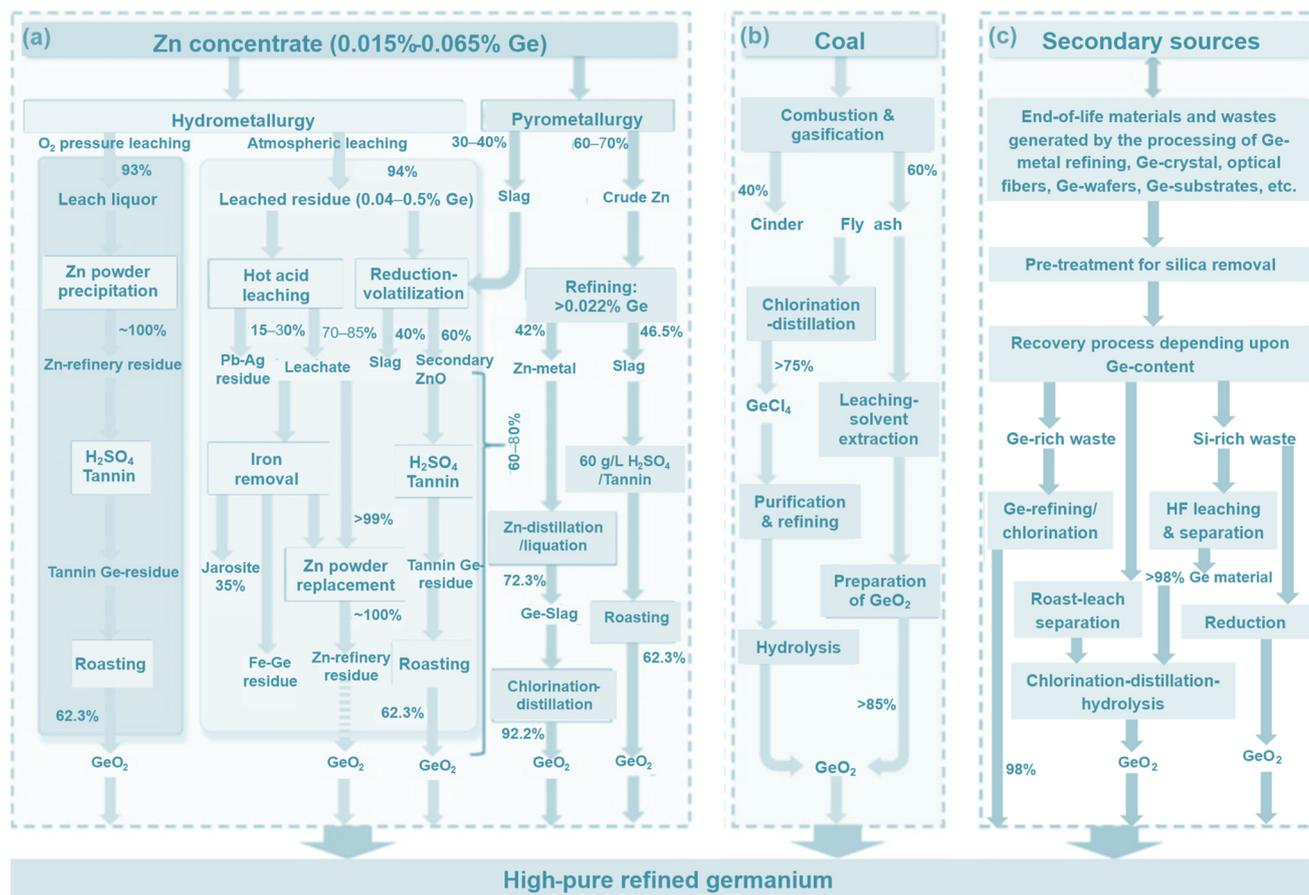
**Fig. 3** Illustration of different processing flow diagrams for germanium extraction from industrial residues of [a] zinc plant mainly through sphalerite ore and [b] coal-burnt fly ash, and [c] via recycling by urban mining end-of-life materials (modified from ref. 26 with permission from Elsevier, *J. Clean. Prod.*, 2021, **294**, 126217, Copyright 2021).
