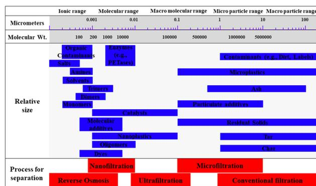
**Fig. 33** Perspectives on the integration of conventional membrane processes in PET recycling: illustration of potential component separations from the outputs of various PET recycling processes.
