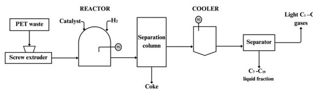
**Fig. 11** Schematic of the hydrocracking/hydrogenation recycling process (adapted with permission.<sup>92</sup> Copyright 2005, Elsevier).
