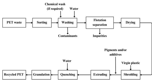
Fig. 6 Schematic of the mechanical recycling process (adapted with permission.<sup>65</sup> Copyright 2009, Elsevier).
