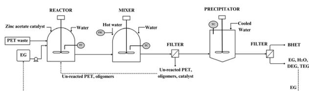
Fig. 12 Schematic of the glycolysis recycling process (adapted with permission.<sup>93</sup> Copyright 2013, Springer Nature).
