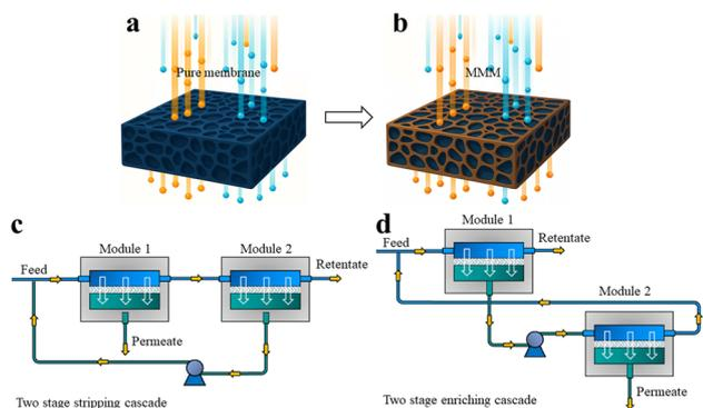
**Fig. 36** Strategies to enhance membrane performance in PET recycling through utilisation of MMMs and implementation of HMSs: (a) pure membrane, (b) MMM, (c) two-stage stripping cascade, and (d) two-stage enriching cascade. (Images for a and b): adapted with permission.<sup>273</sup> Copyright 2023, Elsevier; (images for c and d): adapted with permission.<sup>274</sup> Copyright 2019, IWA Publishing.
