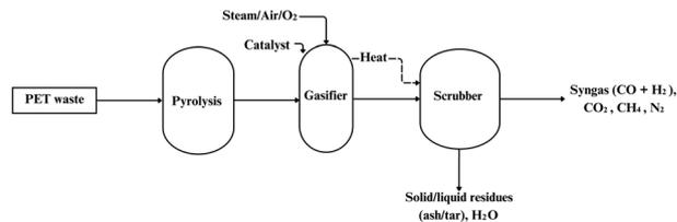
**Fig. 10** Schematic of the gasification recycling process (adapted under terms of the CC-BY license.<sup>88</sup> Copyright 2022, MDPI).
