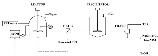
Fig. 24 Schematic of the alkaline hydrolysis recycling process (adapted with permission.<sup>93</sup> Copyright 2013, Springer Nature).
