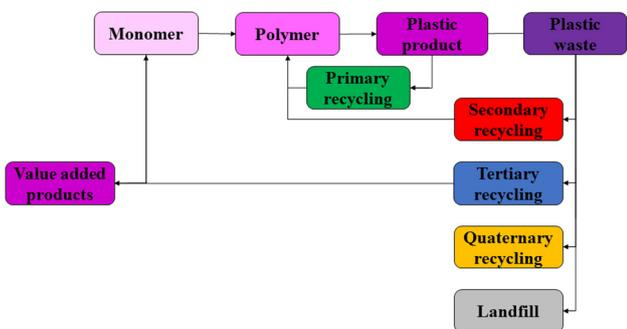
Fig. 3 PET valorisation routes, associated plastic quality, and their position within the processing line (adapted under terms of the CC-BY license.<sup>52</sup> Copyright 2013, Scientific Research Publishing Inc.).
