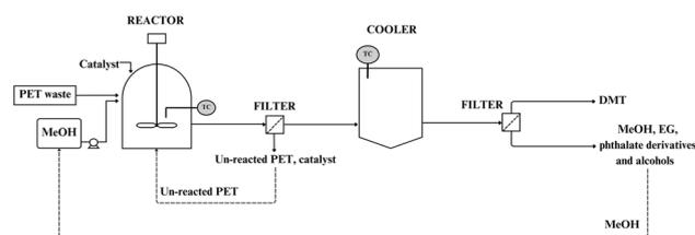
Fig. 14 Proposed schematic of the methanolysis recycling process (based on provided information in ref. 29).
