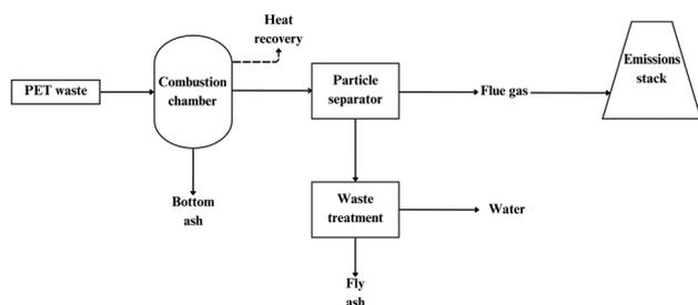
**Fig. 32** Schematic of the incineration recycling process (adapted under terms of the CC-BY license.<sup>126</sup> Copyright 2018, Faculty of Engineering of Nnamdi Azikiwe University).
