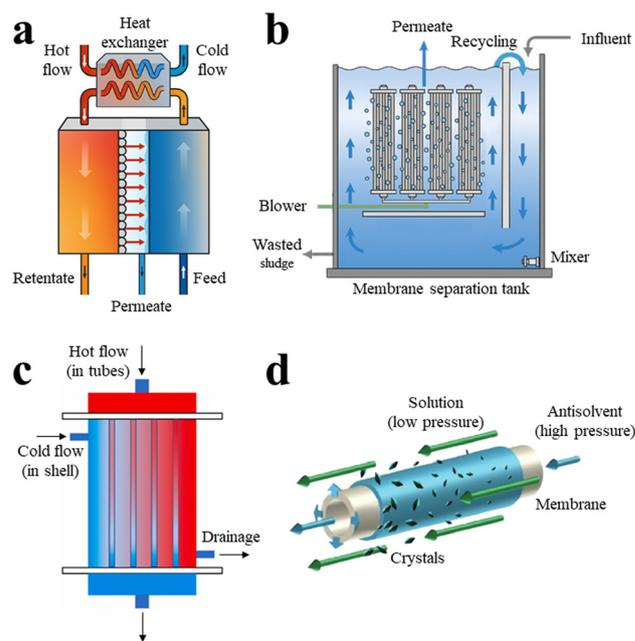
**Fig. 35** Perspectives on the integration of specialised membrane applications in PET recycling, illustrating membrane schematics for: (a) MD, (b) MBR, (c) MHE, and (d) MCr (image for a): adapted with permission.<sup>225</sup> Copyright 2021, Elsevier; image for (b): adapted with permission.<sup>225</sup> Copyright 2015, MDPI; image for (c): adapted with permission.<sup>216</sup> Copyright 2023, Elsevier; image for (d): adapted with permission.<sup>220</sup> Copyright 2023, RSC.
