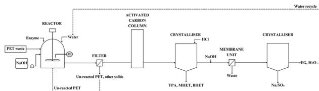
Fig. 26 Schematic of the enzymatic recycling process (adapted with permission.<sup>114</sup> Copyright 2021, Elsevier).
