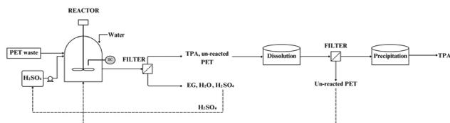
Fig. 20 Proposed schematic of the acidic hydrolysis recycling process (based on provided information in ref. 93 and 100).
