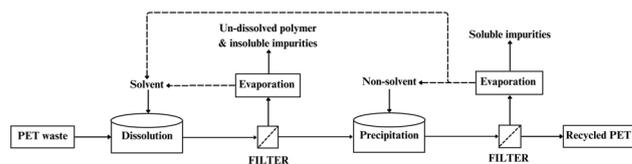
Fig. 7 Schematic of the dissolution recycling process (adapted under terms of the CC-BY license.<sup>69</sup> Copyright 2021, MDPI).
