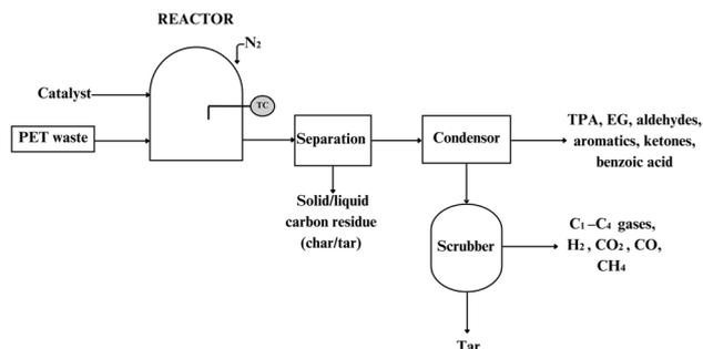
**Fig. 8** Schematic of the pyrolysis recycling process (adapted under terms of the CC-BY license.<sup>80</sup> Copyright 2021, MDPI and CC-BY license.<sup>83</sup> Copyright 2022, Springer Nature).
