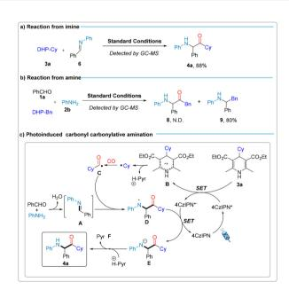
Scheme 4 Photoinduced four-component carbonyl carbonylative amination.
