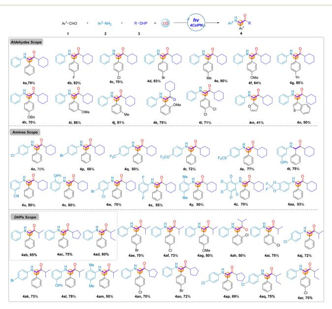
Scheme 1 Substrate scope. Reaction conditions: 1 (0.2 mmol), 2 (0.2 mmol), 3 (0.3 mmol), CHCl<sub>3</sub> (2.0 mL), CO (50 bar), 4CzIPN (5 mol%), under 400–500 nm irradiation, at 30 °C for 24 h. Isolated yield.
