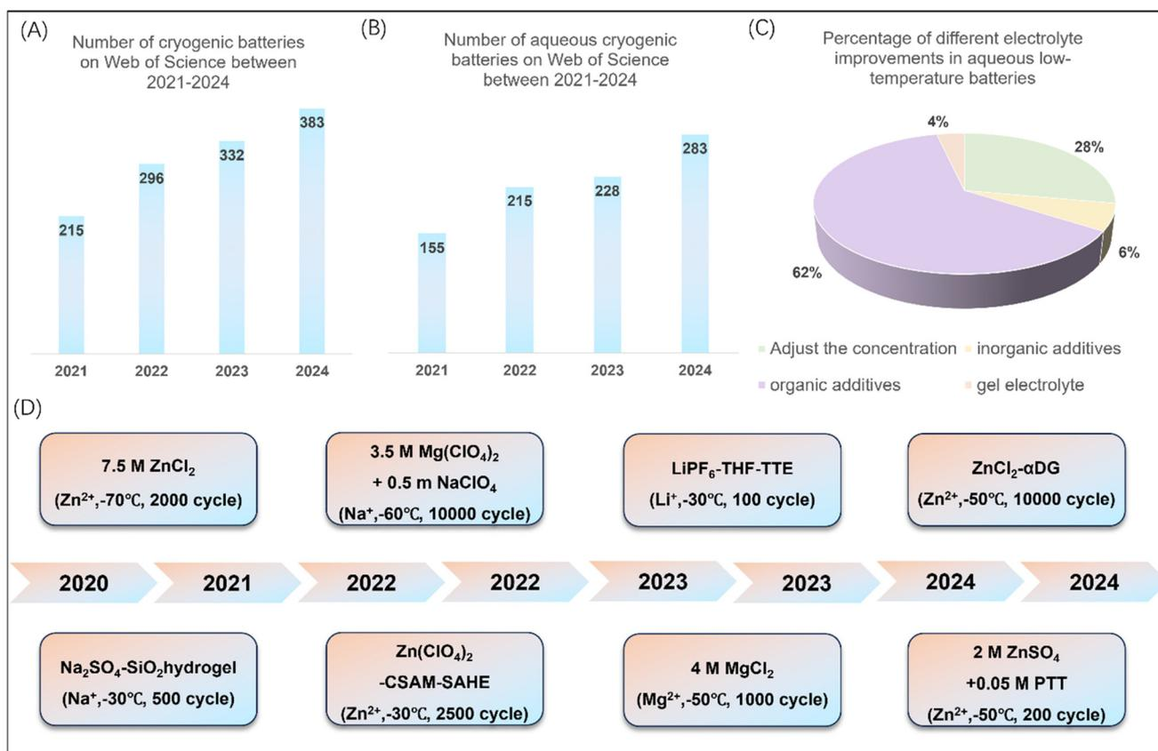
**Fig. 1** (A) Number of low temperature batteries on web of science 2021–2024. (B) Number of low temperature aqueous batteries on web of science 2021–2024. (C) Percentage of different additive categories in low-temperature aqueous batteries. (D) Development of low-temperature water-based batteries in 2020–2024.
