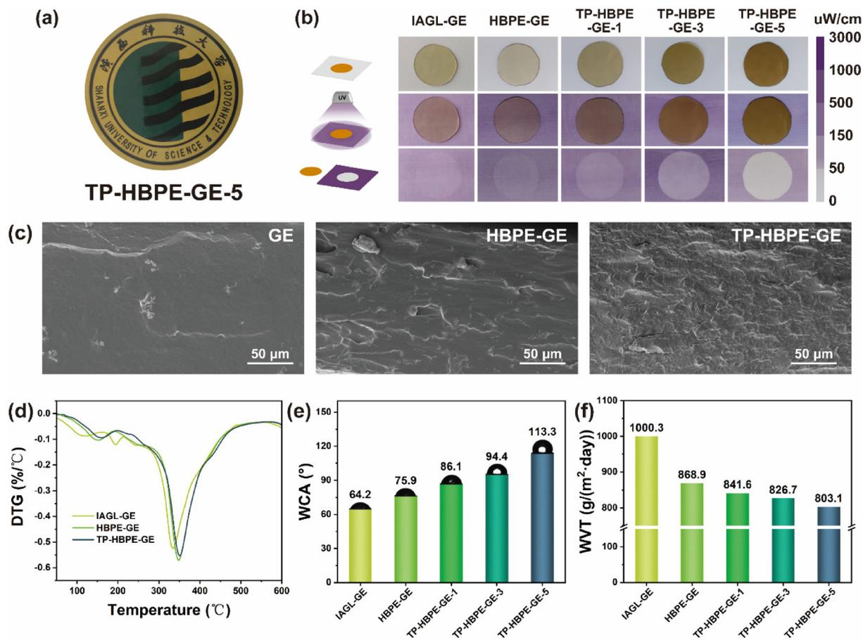
**Fig. 4** (a) Optical images of TP-HBPE-GE-5. (b) Images of UV indicator cards before and after UV exposure for the following films: IAGL-GE, HBPE-GE, TP-HBPE-GE-1, TP-HBPE-GE-3, and TP-HBPE-GE-5. (c) SEM images of IAGL-GE, HBPE-GE, and TP-HBPE-GE-5 films. (d) DTG curves of IAGL-GE, HBPE-GE, and TP-HBPE-GE films. (e) Water contact angles (WCA) and (f) water vapor transmission rates (WVT) of IAGL-GE, HBPE-GE, TP-HBPE-GE-1, TP-HBPE-GE-3, and TP-HBPE-GE-5 films.
