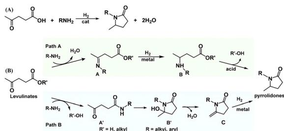
**Scheme 11** (A) Traditional method for synthesizing pyrrolidone from acetoacetic acid and primary amines; (B) two potential pathways for pyrrolidone formation mechanisms.<sup>108,109</sup>
