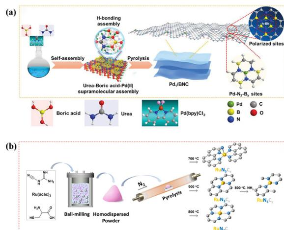
Fig. 13 (a) Schematic of Pd<sub>1</sub>/BNC single-atom catalyst synthesis; (b) schematic of the synthesis of Ru<sub>1</sub>/NC single-atom catalyst supported on nitrogen-doped carbon.<sup>46,148</sup>
