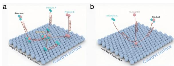
Fig. 6 Mechanisms of reactant conversion to products in multiphase catalytic processes: (a) LH; (b) ER.<sup>129</sup>
