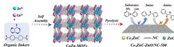
**Fig. 14** Schematic of the synthesis strategy for Co<sub>3</sub>ZnC–ZnO/NC-500 catalyst derived from Co/Zn bimetallic MOF.<sup>177</sup>
