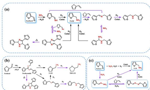
**Scheme 9** Catalytic reductive amination reaction networks of FF.<sup>7,104,105</sup>
