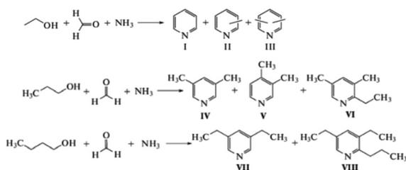
**Scheme 4** Catalytic conversion of formaldehyde and ammonia to six-membered heterocycle pyridine and its derivatives.<sup>82</sup>
