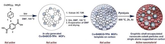
**Fig. 11** MOF-derived Co-DABCO-TPA@C-800 catalyst with Co nanoparticles and single atoms.<sup>172</sup>
