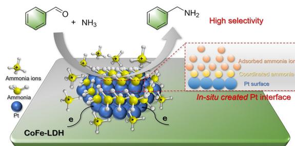
**Fig. 9** *In situ* reconstruction of Pt interface and its coordination ions with ammonia.<sup>156</sup>
