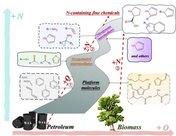
**Fig. 4** Simplified routes to NCCs from petroleum and biomass resources. ① “+O”: oxidation or dehydrogenation of petroleum hydrocarbons to oxygenates (Cu, Pd, acid catalysts, 200–350 °C); ② “+N”: amination/cyclization of oxygenates to NCCs (NH<sub>3</sub>, Ni, Ru, HZSM-5, 300–500 °C); ③ “+N”: biomass undergoes direct N-rich pyrolysis to form NCCs in one step (urea or NH<sub>3</sub> co-feeding, 400–600 °C).
