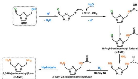
**Scheme 13** Amination of HMF to BAMF conversion via distributed catalysis using RANEY® Ni.<sup>171</sup>
