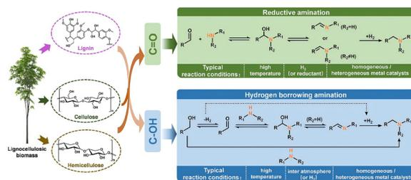
**Scheme 2** The primary pathways for thermocatalytic amination of biomass-based compounds.<sup>12</sup>
