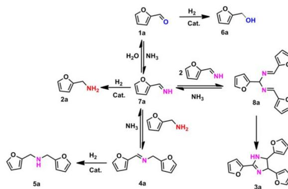
**Scheme 12** FF reduction amination to FAM and potential side reactions.<sup>148</sup>
