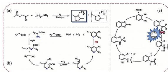
**Scheme 6** (a) Conversion of biomass-derived 2,5-hexanedione into *N*-substituted tetrahydropyrroles using Ru-based catalysts; (b) decarboxylative oxidation and cyclization of amino acids and aldehydes to form pyridine; (c) synthesis of NHCs from aniline and its derivatives with aldehydes.<sup>99–101</sup>
