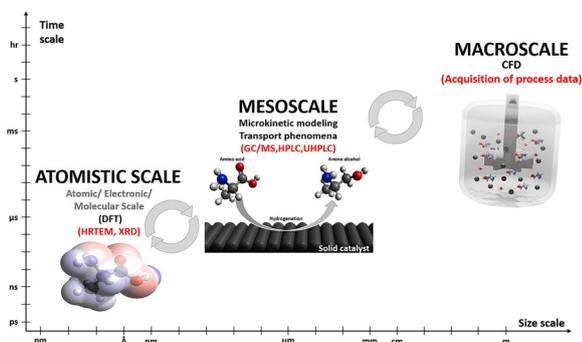
**Fig. 5** Multiscale modeling approaches in the production of high-value NCCs.<sup>116</sup>
