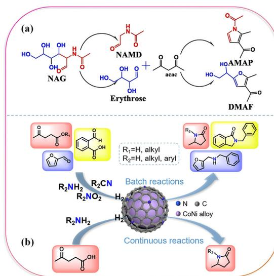
**Scheme 10** (a) Catalytic retro-aldol reaction of NAG to form furan and pyrrole derivatives; (b) continuous and stable reductive amination of acetoacetic acid with amines.<sup>106,107</sup>
