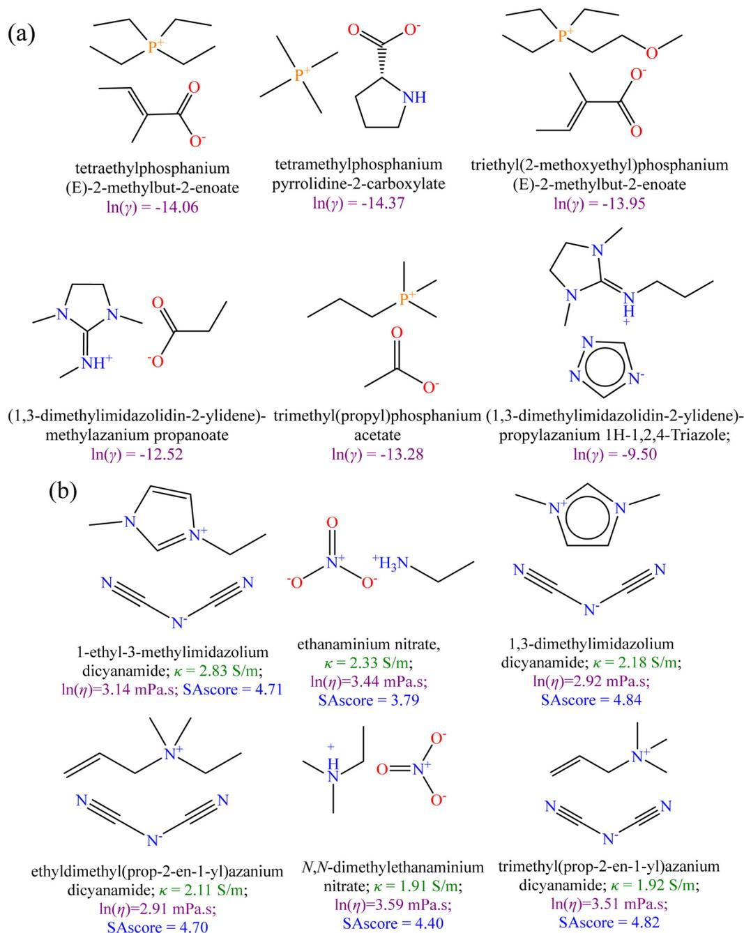
**Fig. 9** (a) COSMO-RS predicted logarithmic activity coefficient of lignin in ML developed ionic liquids. (b) Ionic conductivity of newly engineered ionic liquids for battery research applications. All these ILs are predicted to be easy to synthesize with a SA score below 6.
