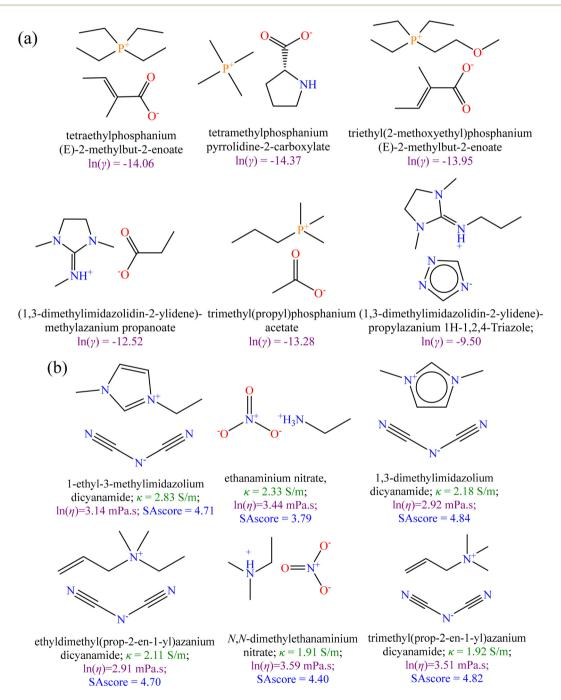
Fig. 9 (a) COSMO-RS predicted logarithmic activity coefficient of lignin in ML developed ionic liquids. (b) Ionic conductivity of newly engineered ionic liquids for battery research applications. All these ILs are predicted to be easy to synthesize with a SA score below 6.
