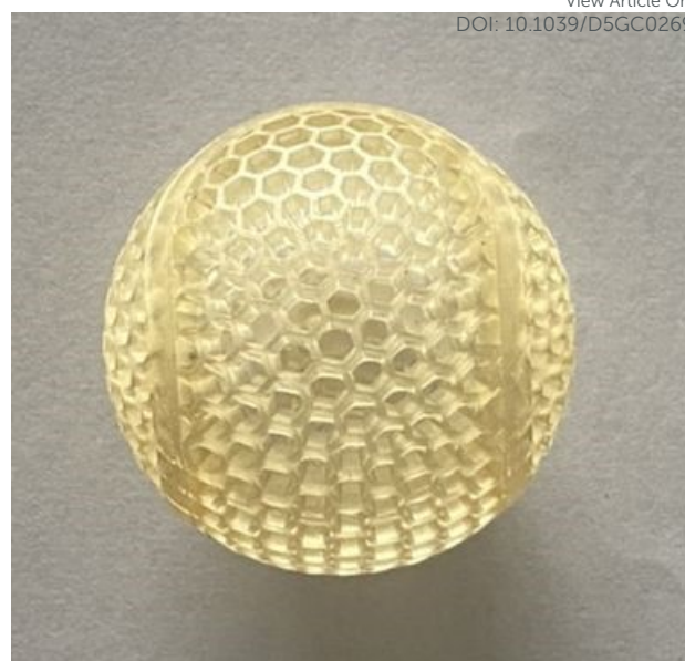
Figure 5. Honeycomb-patterned hollow tennis ball printed with 75% PDHIA_0.5, thus containing 22 wt.% of recycled PET. Object diameter is 40 mm.
