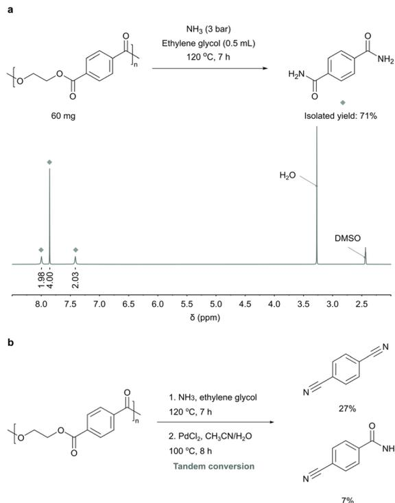
**Fig. 4** (a) Ammonolysis of PET and the NMR spectrum of the product. (b) Tandem conversion of PET into terephthalonitrile. Reaction conditions for ammonolysis (step 1): PET (60 mg), ethylene glycol (0.5 mL), ammonia (3 bar, charged at  $-20$  °C), 120 °C, 7 h. Reaction conditions for dehydration (step 2): product from step 1, PdCl<sub>2</sub> (6 mg), CH<sub>3</sub>CN (3 mL), H<sub>2</sub>O (3 mL), 100 °C, 8 h.
