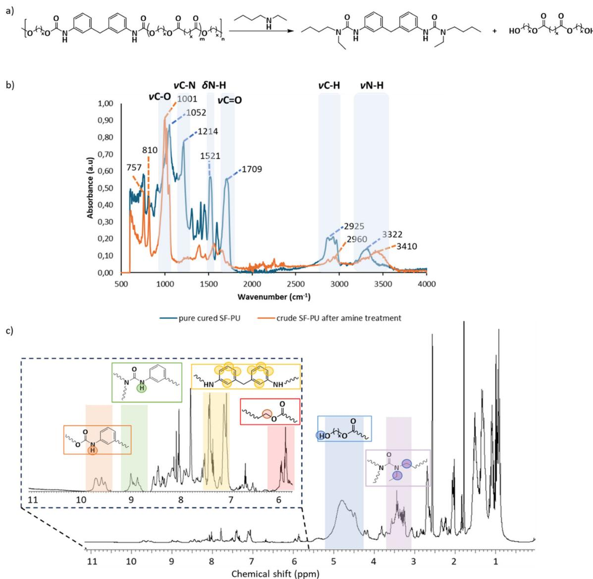
**Fig. 2** (a) Chemical reaction scheme of aromatic polyester polyurethane (PU) with *N*-ethyl *N*-butyl amine (EBA); (b) FTIR spectra of the aromatic polyester polyurethane (PU) adhesive before and after EBA treatment; (c) NMR spectrum of the aromatic polyester polyurethane (PU) adhesive after EBA treatment.
