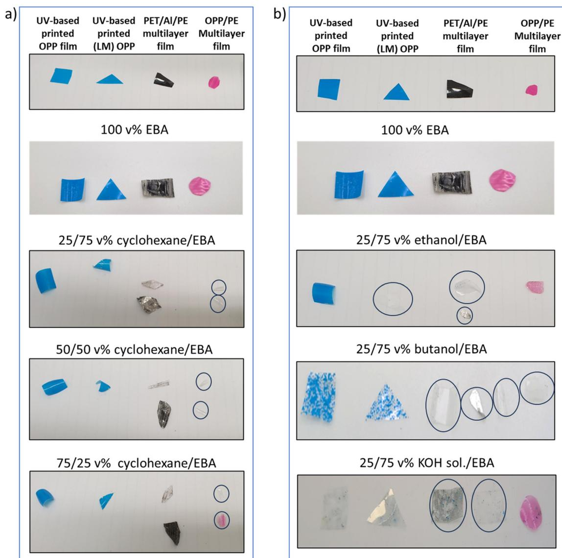
**Fig. 5** Deinking and delamination of 4 different plastic films (a) in cyclohexane/*N*-ethyl *N*-butyl amine (EBA) mixture at different volume ratios; (b) in ethanol/EBA, butanol/EBA and KOH solution/EBA mixtures at 25/75 v% ratio after 4 h contact at 60 °C. Hourly visual progression of deinking and delamination of these samples in each medium is given in Fig. S5.
