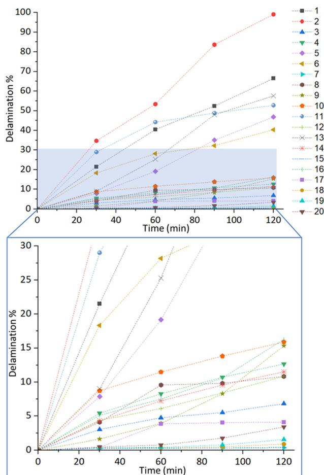
**Fig. 3** Experimental kinetic data of delamination of the violet colored PET/PE multilayer sample (sample 7) through selective aminolysis of the adhesive in *N*-ethyl *N*-butyl amine (EBA) during 120 minutes. Detailed experimental data points are given in the SI, Table S2. The data points are connected with dashed lines for easier visualization. The standard deviation of delamination %, based on the 6 center points of DoE, is 5.97%.
