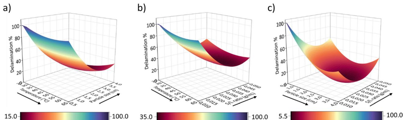
**Fig. 4** Response surfaces of the delamination % as a function of (a) temperature (°C) and particle size (cm); (b) temperature (°C) and S/L ratio (g mL<sup>-1</sup>); (c) particle size (cm) and S/L ratio (g mL<sup>-1</sup>) for delamination of sample 7 through selective aminolysis of the PU adhesive layer. Delamination percentages exceeding 100% fall within the experimental error margin of the RSM model and are normalized to 100%.
