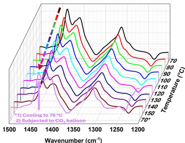
Fig. 2 3D *in situ* ATR-FTIR partial spectra (absorbance vs. wavenumber vs. temperature) of the MCA adduct dissolved in DMSO. The solution was heated from 70 to 150 °C, then cooled back to 70 °C before being exposed to CO<sub>2</sub> via a balloon.
