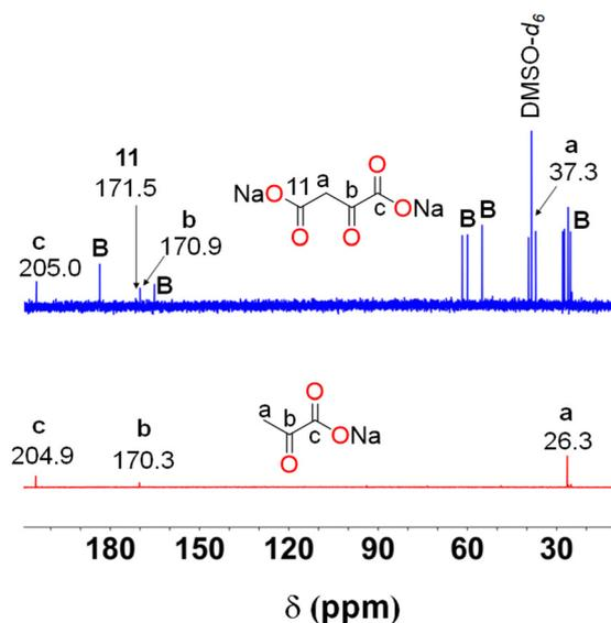
**Fig. 4**  $^{13}\text{C}$  NMR spectra of sodium pyruvate (red trace) and SOA (blue trace) measured in  $\text{D}_2\text{O}$ . B: labels corresponding to the biotin peaks. The carbon labeled as 11 in SOA corresponds to the carbon atom transferred from BCCA.
