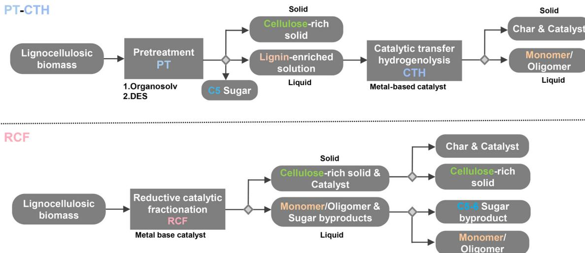
**Fig. 1** Process flow of PT-CTH and RCF biorefinery processes. Color codes of the concerned processes and substrates used throughout this article: light blue: pretreatment followed by catalytic transfer hydrogenation (CTH); pink: reductive catalytic fractionation (RCF); green: cellulose; dark blue: mono sugar products; orange: lignin and its monomer product.
