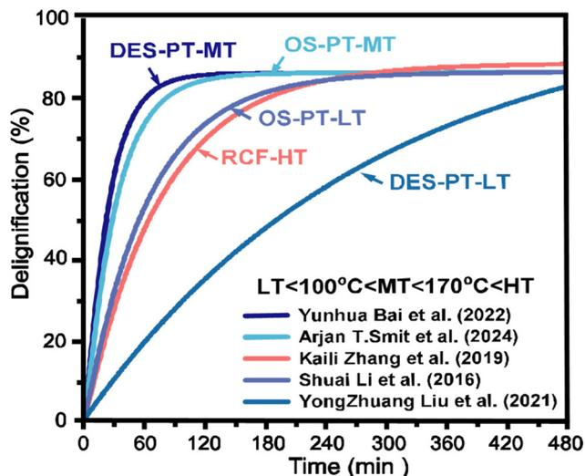
Fig. 8 Delignification kinetics in various pretreatment methods and RCF (Appendix 6 in the SI).<sup>26,120,121,169,171</sup>
