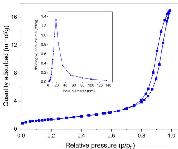
Fig. 4  $N_2$  isotherm curve of the malate material. The inset shows the BJH pore size distribution.
