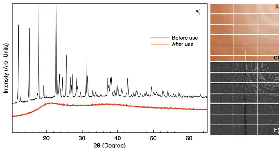
Fig. 5 (a) XRD patterns of the malate material before (black line) and after (red line) the photothermo-catalytic tests. Before the functional test, all the peaks in the XRD pattern can be attributed to the newly detected phase  $\text{MH}_2(\text{C}_4\text{H}_4\text{O}_5)_2 \cdot 4\text{H}_2\text{O}$ , with M representing the metals. 2D images of XRD patterns of the malate phase (b) before and (c) after photocatalytic tests collected under synchrotron radiation are also shown.
