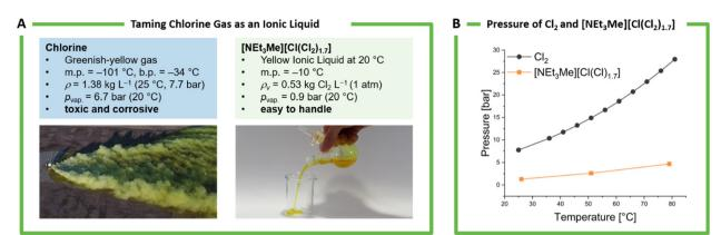
Fig. 2 Physical properties of elemental chlorine in comparison to the ionic liquid [NEt<sub>3</sub>Me][Cl(Cl<sub>2</sub>)<sub>1.7</sub>] (A) and the temperature-dependent pressure of elemental chlorine in comparison to the ionic liquid [NEt<sub>3</sub>Me][Cl(Cl<sub>2</sub>)<sub>1.7</sub>] (B).
